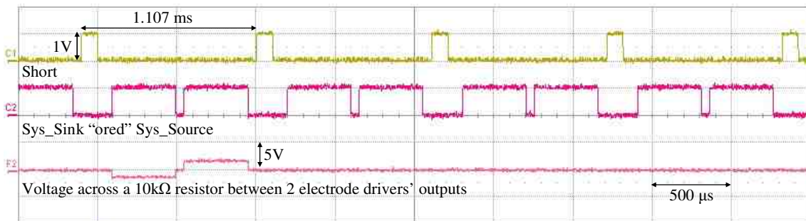
Figure 90 Measurement result with time slice = 1.107 ms and pulse width = 400 \mu s
