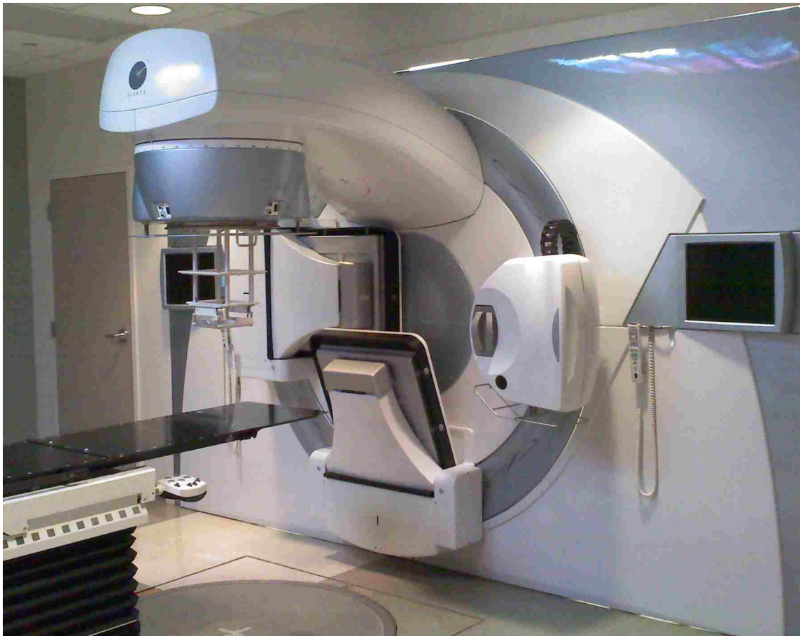
Figure 2.1: Elekta Infinity series linear accelerator in electron mode. Note the wall-mounted gantry with the 14 \times 14 \text{ cm}^2 applicator attached and that the imaging components are retracted during electron mode.
