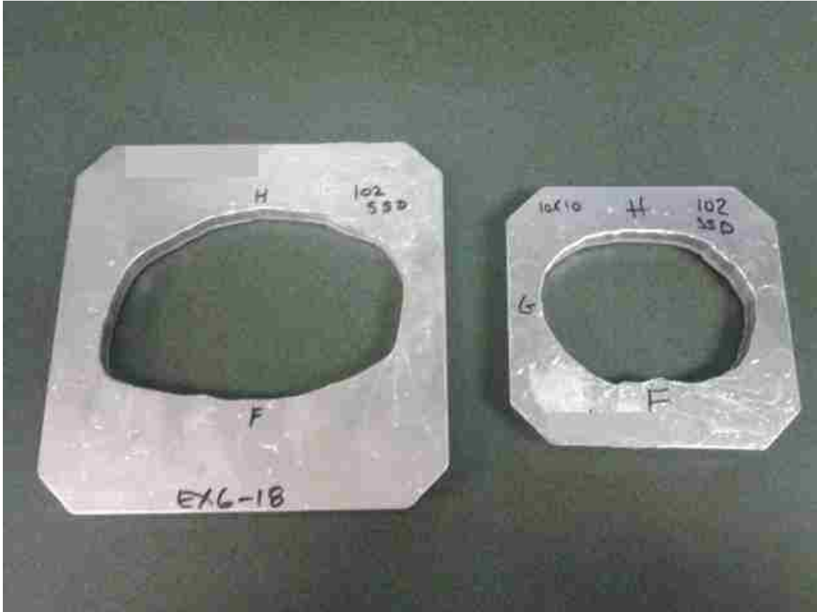
Figure 1.4: Two custom Cerrobend inserts shaped to a patient's PTV. The insert on the left is for a 15x15 cm 2 applicator while the insert on the right is for a 10x10 cm 2 applicator.
