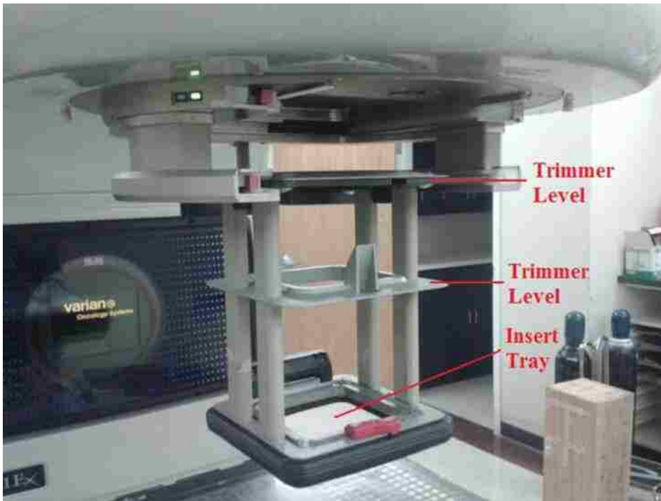
Figure 1.3: Type III Varian electron applicator with labels showing the trimmers and tray for placement of patient-specific inserts.
