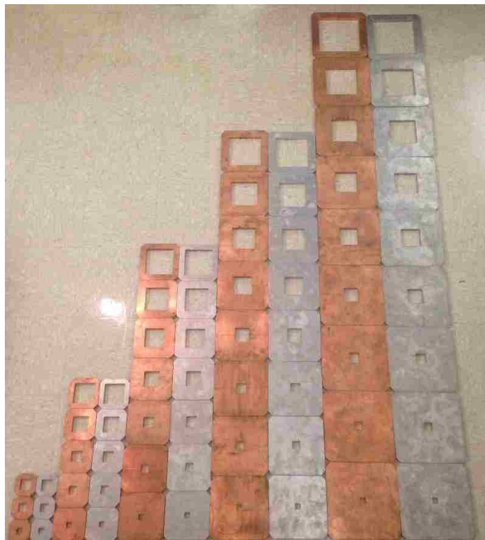
Figure 2.2: Full set of 32 matching pairs of copper and Cerrobend inserts. From left to right: 3, 5, 7, 8, and 9 pairs of inserts for the 6x6 cm 2 , 10x10 cm 2 , 15x15 cm 2 , 20x20 cm 2 , and 25x25 cm 2 applicators, respectively.
