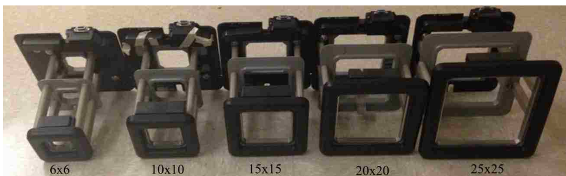
Figure 2.3: All five Varian Type III electron applicators. Pictured from left: 6x6 cm 2 , 10x10 cm 2 , 15x15 cm 2 , 20x20 cm 2 , and 25x25 cm 2 applicators.
