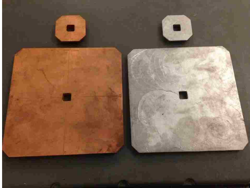
Figure 3.8: Matching copper (left) and Cerrobend (right) 2x2 cm 2 field size inserts for a 6x6 cm 2 applicator (top) and a 25x25 cm 2 applicator (bottom). The larger applicator insert has 621 cm 2 surface area while the smaller applicator insert has 32 cm 2 surface area.
