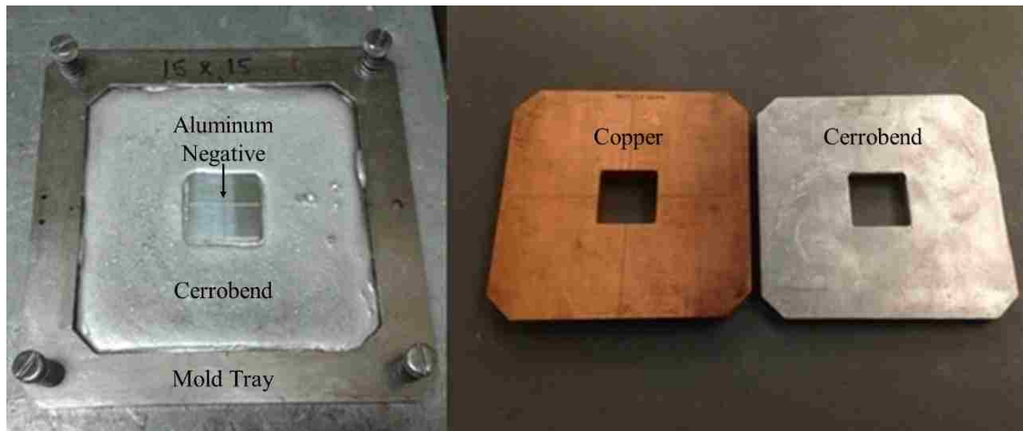
Figure 2.1: (LEFT) Photo of Cerrobend poured into a 15x15 cm 2 applicator mold to generate an insert formed by a 4x4 cm 2 aluminum negative. (RIGHT) The resulting Cerrobend insert alongside its matching copper insert.
