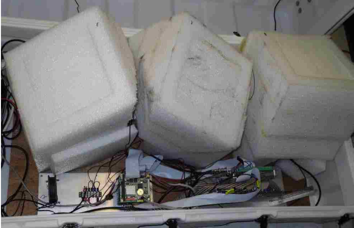
Figure 3.3 Inside a TETRA detection box. The three foam blocks house the NaI PMTs described above. The electronics boards are located at the bottom right. The PC104 stack is located at the bottom left. Power and Ethernet cabling is to the left (not shown).
