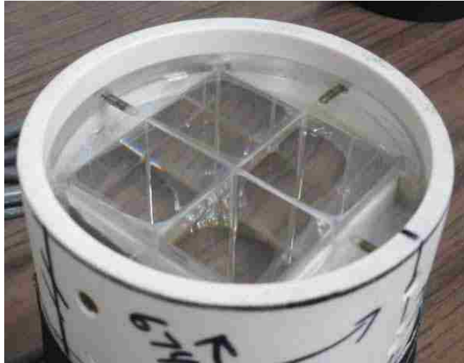
Figure 7.1 2 x 2 BGO scintillator array mounted in 4" PVC.
