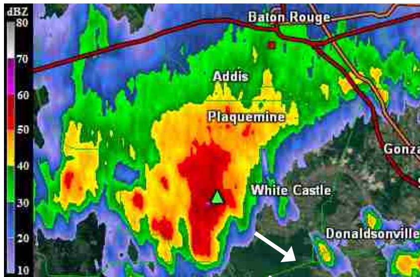
Figure 6.2 Smoothed radar image of the single cell thunderstorm producing the TETRA TGF on 12 Mar 2012. Colors in the image correlate to the density of the cloud in decibels at the lowest elevation angle ( 0.5^\circ ) as indicated in the scale at left. The white arrow indicates the direction of storm movement. The green triangle indicates the location of hail. The red square near the top of the figure is the location of TETRA. Local interstates and highways are shown with red and orange lines near the top of the image. The locations of various cities are also labeled for reference. The image is approximately 90 km by 50 km.
