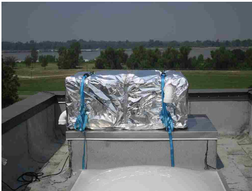
Figure 3.1 One of the four TETRA detector boxes. The boxes are covered with Mylar to reflect ultraviolet (UV) radiation. The PVC curved pipes shown are to promote air flow through the box. This box is located on the roof of the LSU School of Veterinary Medicine. The Mississippi River can be seen in the background.
