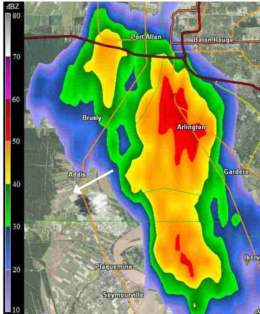
Figure 6.6 Smoothed radar image of the storm producing two TETRA TGFs on 22 Jun 2013. Image was taken at the time of the first TETRA TGF. Colors in the image correlate to the density of the cloud in decibels at the lowest elevation angle as indicated in the scale at left. The white arrow indicates the direction of storm movement. The red square is the location of TETRA. Local interstates and highways are shown with red and orange lines near the top of the image. The locations of various cities are also labeled for reference. The image is approximately 25 km by 40 km.
