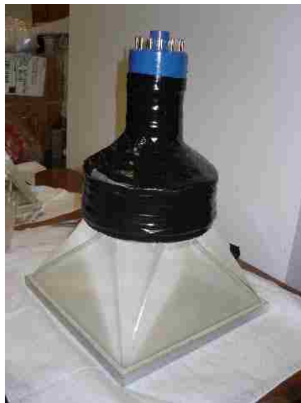
Figure 3.4 One of TETRA's NaI PMT assemblies. The 19 cm x 19 cm x 5 mm NaI(Tl) scintillator is shown at the bottom of the assembly. The clear prism in the middle is the acrylic light guide described above. A 130mm PMT views the light guide from the top, shown wrapped in electrical tape. This assembly is turned upside-down in the detection box to view gamma rays from thunderstorms.
