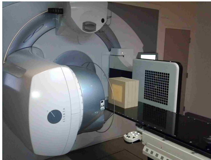
Figure 2.9. Setup for the beam delivery for the Elekta linac with iView EPID. All beams for this study were delivered laterally to minimize transmission through the couch.
