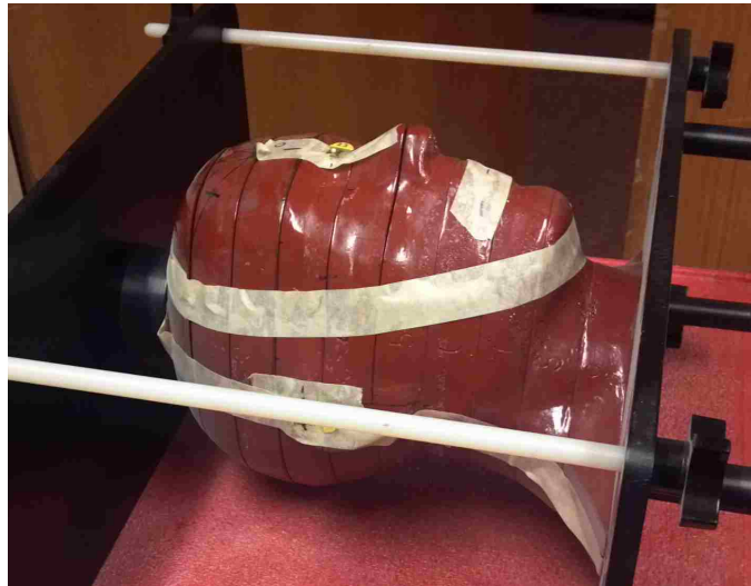
Figure 2.16. Anthropomorphic head phantom used in Aim 4 (RSD Rando ART-210 Head and Neck Phantom, Radiology Support Devices, Long Beach, CA).
