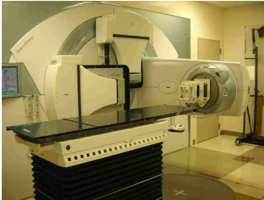
Figure 2.7. Accelerator configuration during irradiation. The accelerator's gantry angle was set to 90^\circ , collimator angle to 0^\circ , and couch angle to 270^\circ to deliver a horizontal beam to the magnetic spectrometer. During irradiation, the Cerrobend ® aperture insert replaced the open-field applicator insert shown here.
