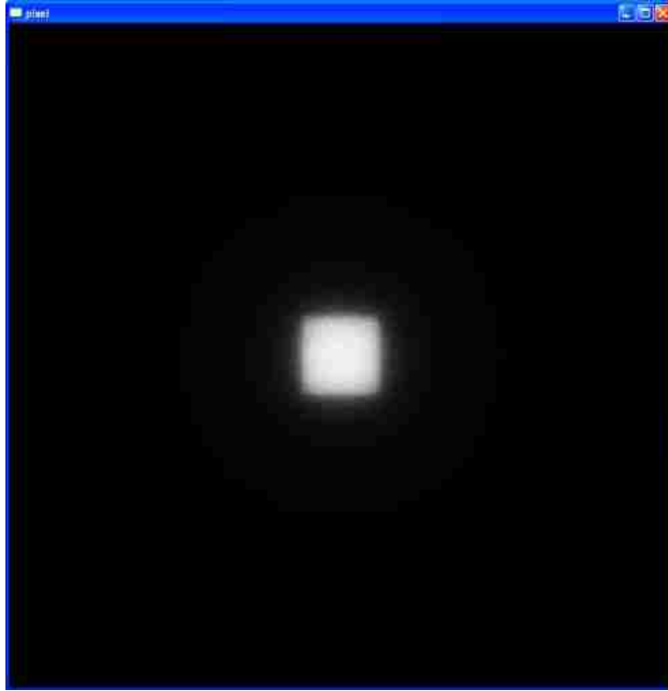
Figure B.2 Image of intensity of final characteristic x-ray absorption position when beam is uniform over a square pixel.
