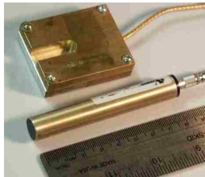
Figure 5.3 Planar detector (top) and capacitive grid detector (bottom). The small size and ability to operate at room temperature make CZT detectors ideal for clinical use.
