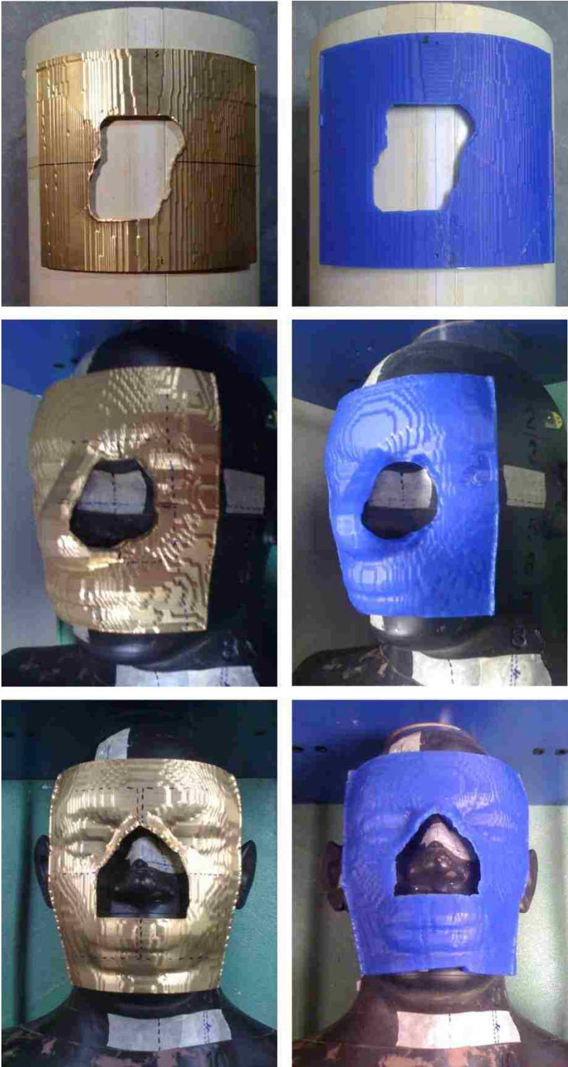
Figure 4.5 (continued): Cylindrical phantom eSC (top row) and the anthropomorphic head phantom case #1 (middle row) and case #2 (bottom row) eSC—[a] brass, Cerrobend, and lead (left to right) and [b] brass (left) and the wax replicas (right).
