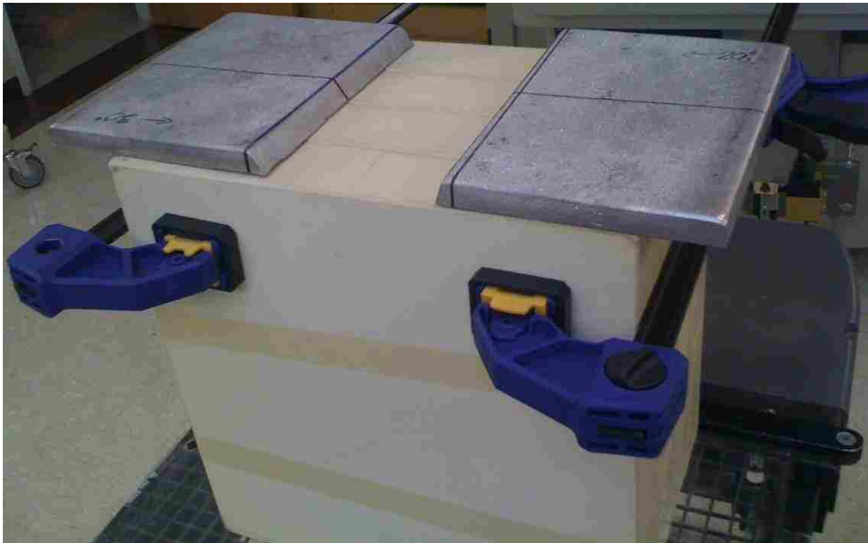
Figure 3.4: Example setup of the phantom apparatus used for bevel angle measurements. The two beveled collimators pictured are the +30^\circ collimator (on left) and the +20^\circ collimator (on right). Each are placed 5 cm from central axis atop four-5 cm slabs of solid water. This image was taken during our preliminary investigation using a 12 MeV beam and including bevel angles up to 30^\circ .
