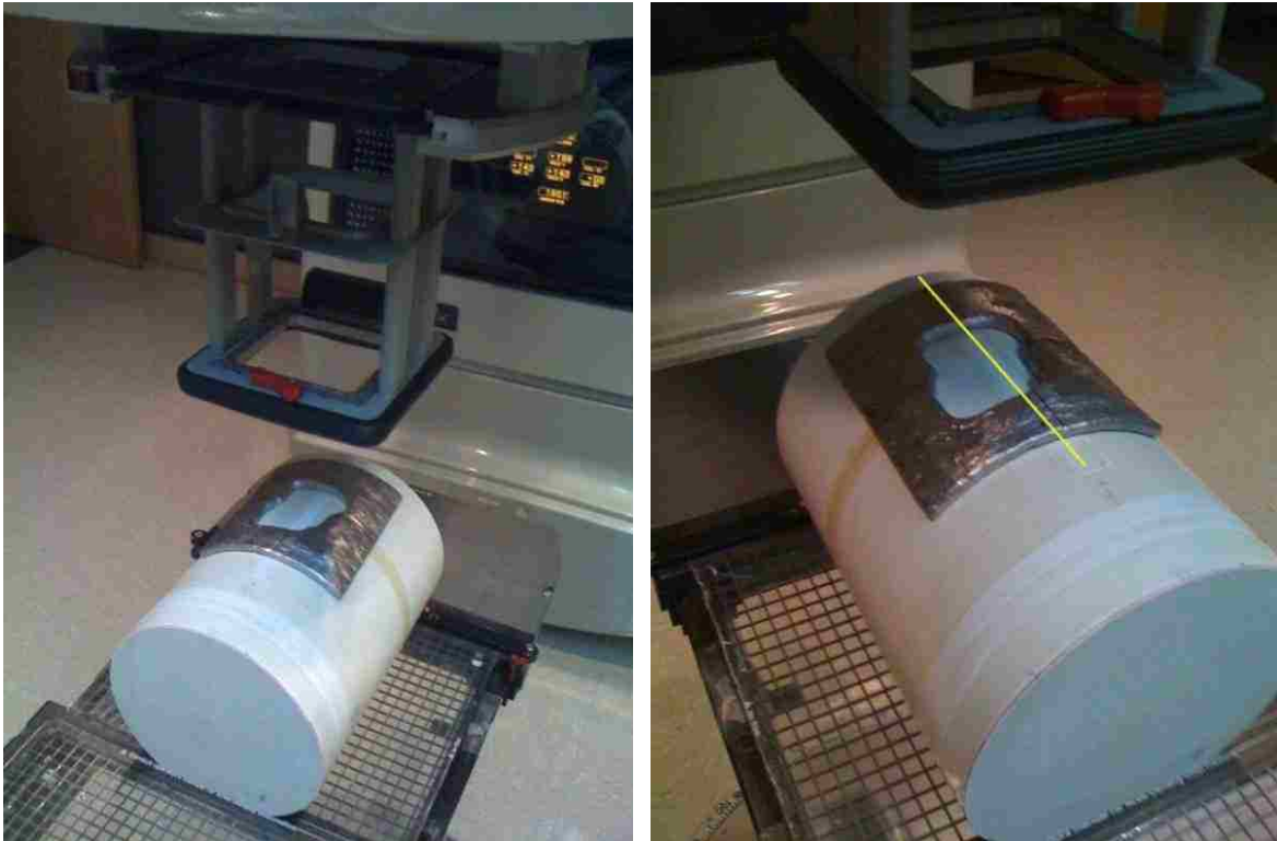
Figure 5.1: Cylindrical phantom experimental setup with Cerrobend eSC, pictured from the foot of the couch. The phantom was extended further from the measurement SSD of 105 cm to allow the view (photo) of the eSC placement. This particular image shows the Cerrobend eSC on the phantom. The couch, gantry, and collimator rotation were all set to 0^\circ . For variation of the gantry from the nominal delivery angle, the couch and collimator were rotated to 90^\circ , and the gantry was set to +3^\circ ; these adjustments allowed for a +3^\circ gantry rotation within the film plane (central sagittal plane). The proximal edge of the film plane is approximated in the right image by a line drawn along the longitudinal surface of the phantom.
