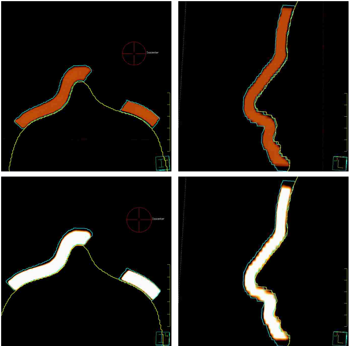
Figure 4.7: kVCT and MVCT fusion images of the head phantom (case #1). Shown are the kVCT images (upper) of the wax eSC replica, where the planned eSC shape is represented by the blue line. A contour of the planned eSC shape is also shown overlaying the MVCT images (lower) of the brass eSC. The images on the left are transverse slices through CAX, and the right images are sagittal slices through the central-sagittal axis of the phantom, which was not parallel to the beam CAX as the beam had a gantry rotation of +40^\circ (see Figure 4.4). For the kVCT of the wax eSC replica, the window and level values used were 1012 and 462, respectively. For the MVCT of the brass eSC, the window and level values used were 1401 and 2599, respectively. For this phantom case, CT images were collected without the use of the head phantom. The blue contour in the images is the external contour of the head phantom. The brass eSC for the first head phantom case corresponded well to the planned eSC. The lone deviation was a shortened brass eSC in the superior-inferior direction. Similar to the cylindrical phantom, this eSC was approximately 5-10 mm short of the full planned superior-inferior length (about 2.5-5.0 mm from each end).
