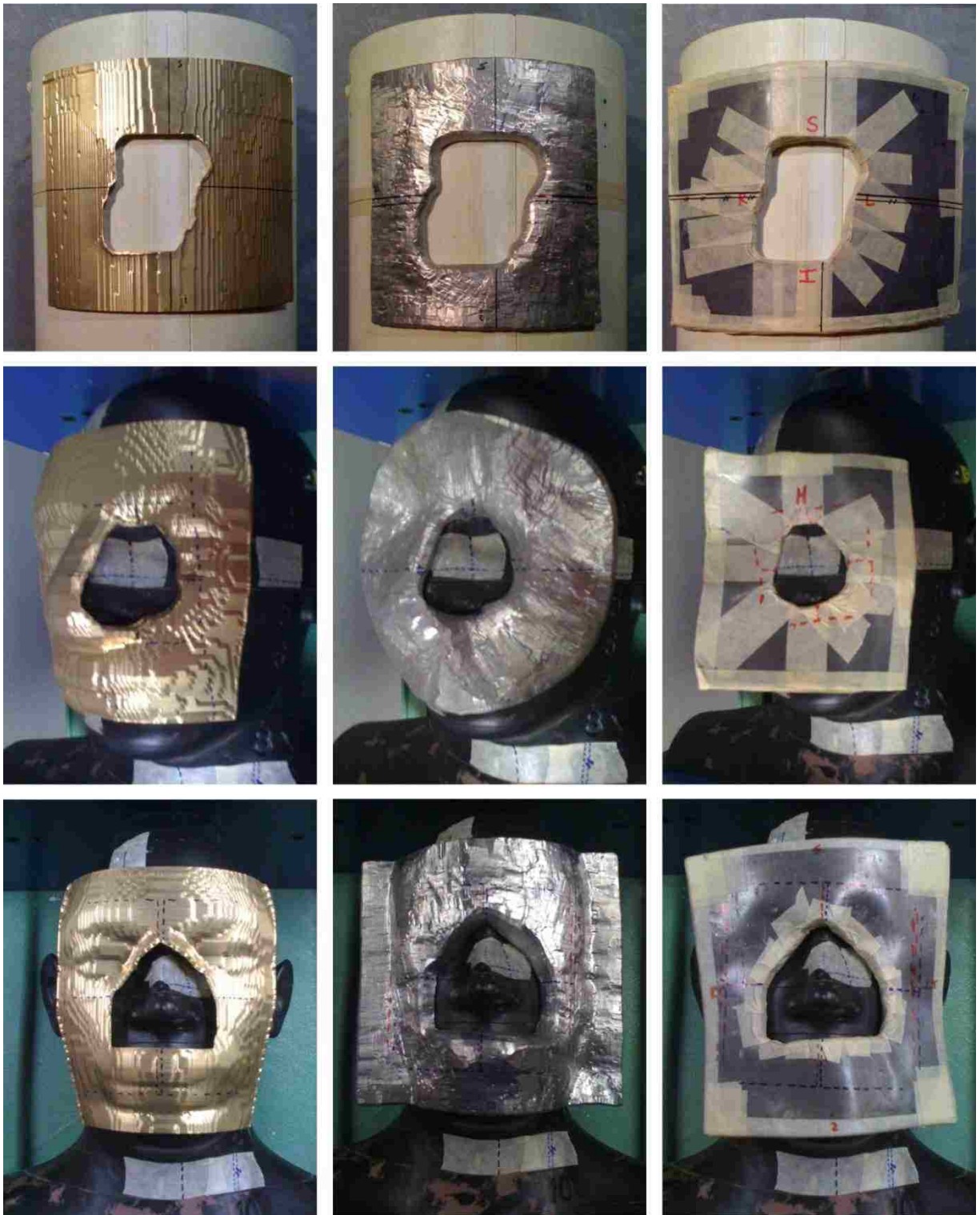
Figure 4.5: Cylindrical phantom eSC (top row) and the anthropomorphic head phantom case #1 (middle row) and case #2 (bottom row) eSC—[a] brass, Cerrobend, and lead (left to right) and [b] brass (left) and the wax replicas (right).
