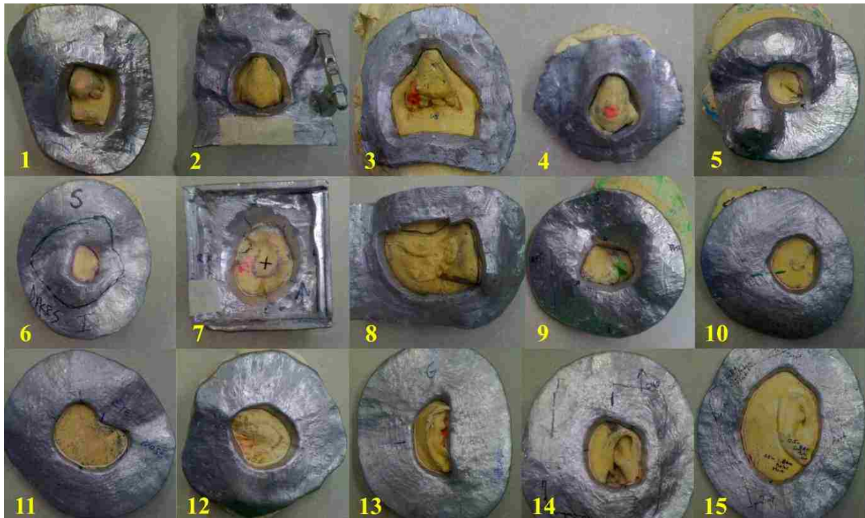
Figure 3.1: Collection of patient Cerrobend skin collimators used to determine common clinical attributes. The general treatment sites are as follows: whole nose (1-4), inner canthus (5), partial nose (6-9), scalp/cheek/forehead (10-12), and ear (13-15).
