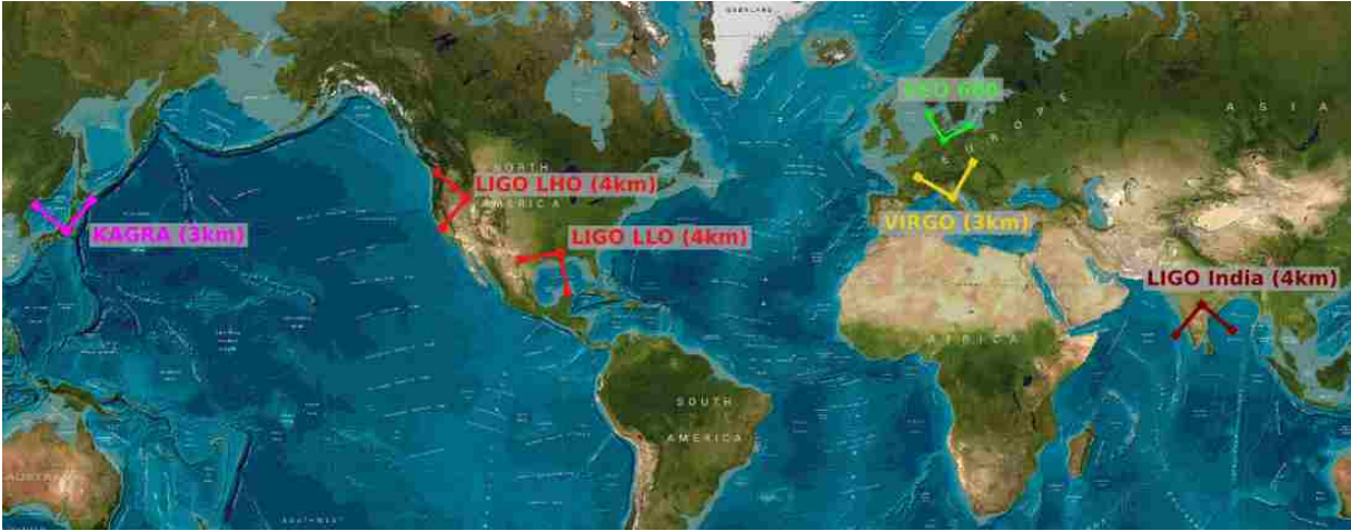
Figure 1.2: Current and planned interferometric GW detectors. The two US LIGO sites, VIRGO and GEO are in operation or in upgrade stages. KAGRA construction in Japan has begun, and will be an underground cryogenic detector. A third LIGO site is planned in India but construction has not begun at the time of this writing.
