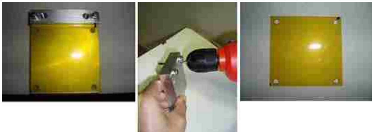
Figure 2.11: Holes were punched in the film so it could be placed in the film block. (Left) Film was placed in the film template, top removed. (Center) Once the top was attached, a drill was used to make four holes in the film. (Right) Resulting film, ready to be placed in the film block.
