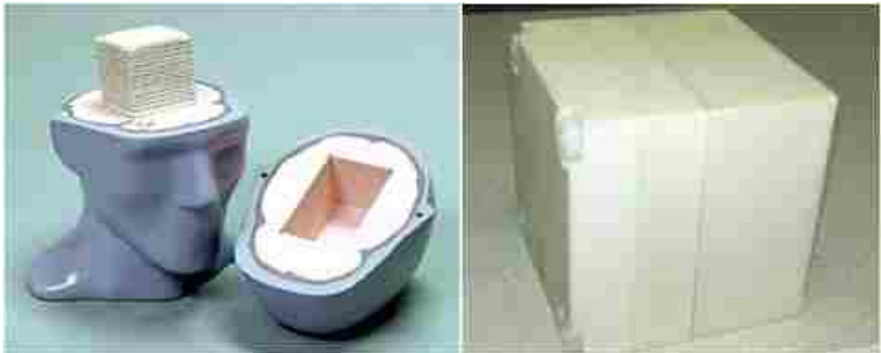
Figure 2.1: (Left) CIRS Model 605 Radiosurgery head phantom. (Right) 6.35x6.35x6.35 cm 3 plastic block to hold up to 2 pieces of x-ray film; Figure 2.13 illustrates the placement of the film within the block.
