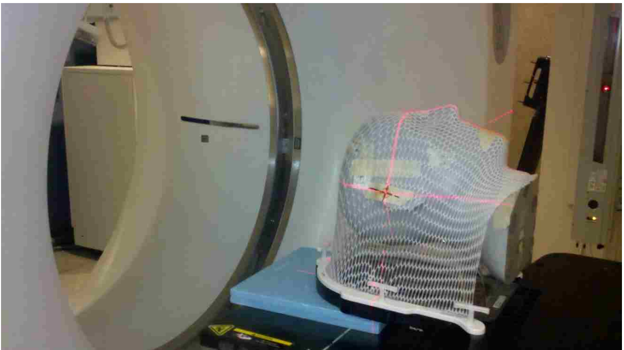
Figure 2.2: Head-phantom setup on the CT couch. In order to get the axial film plane parallel to the CT imaging plane, the head-phantom needed to be tilted upwards using the Styrofoam boards. Radiopaque BB's were placed at the laser crosshairs so setup could be mimicked on the treatment couch.
