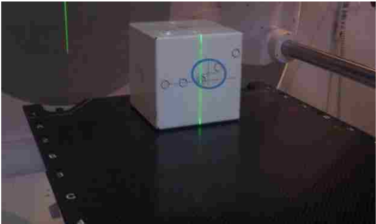
Figure 1.4: Image of the Penta-Guide phantom placed on the Elekta Infinity treatment couch. The phantom is initially setup to the crosshairs that are offset from the center of the cube.
