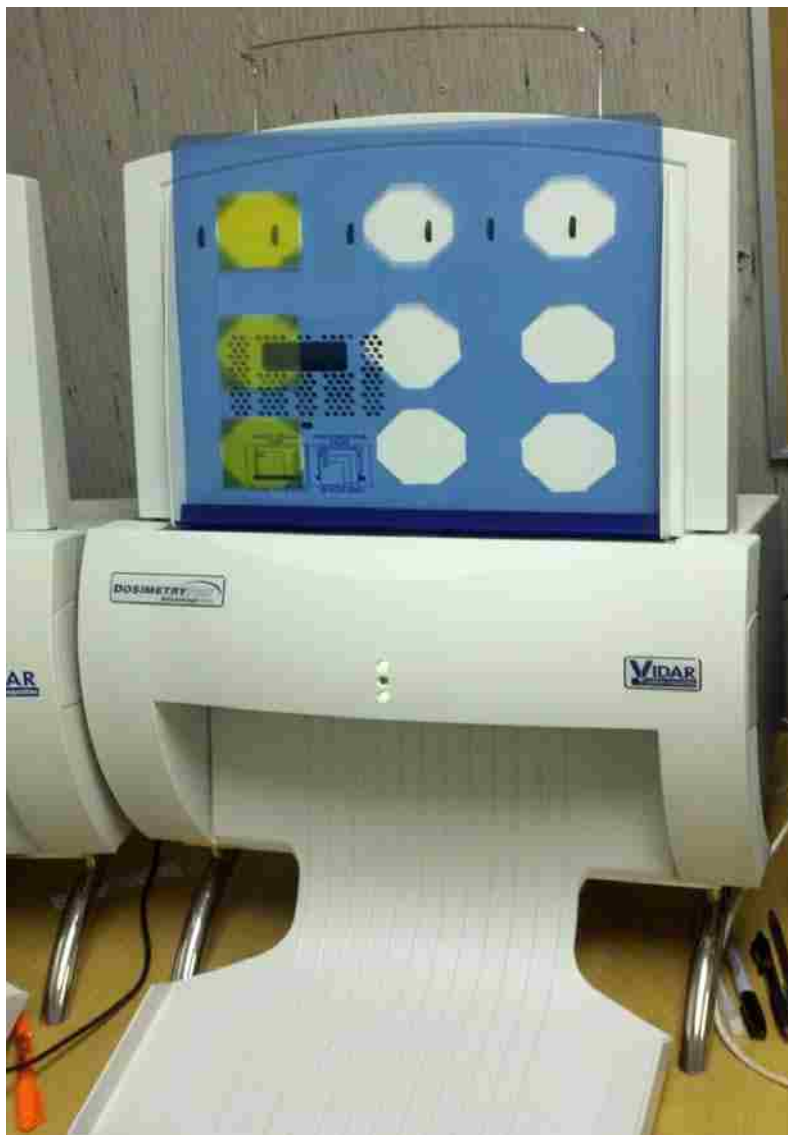
Figure 2.20: Photo of the Vidar DosimetryPRO Advantage(RED) film digitizer and the scanning template used to hold the film squares. Three film pieces (yellow squares) are in place on the template.
