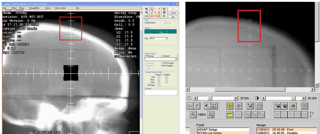
Figure 2.19: (Left) Screen capture of the Right-Lateral DRR acquired from the Pinnacle 3 treatment plan; the tick marks on the horizontal and vertical axes represent 1 cm intervals in the plane of isocenter. (Right) Screen capture of the corresponding MV port film. The white dots denote 1 cm intervals in the plane of isocenter.
