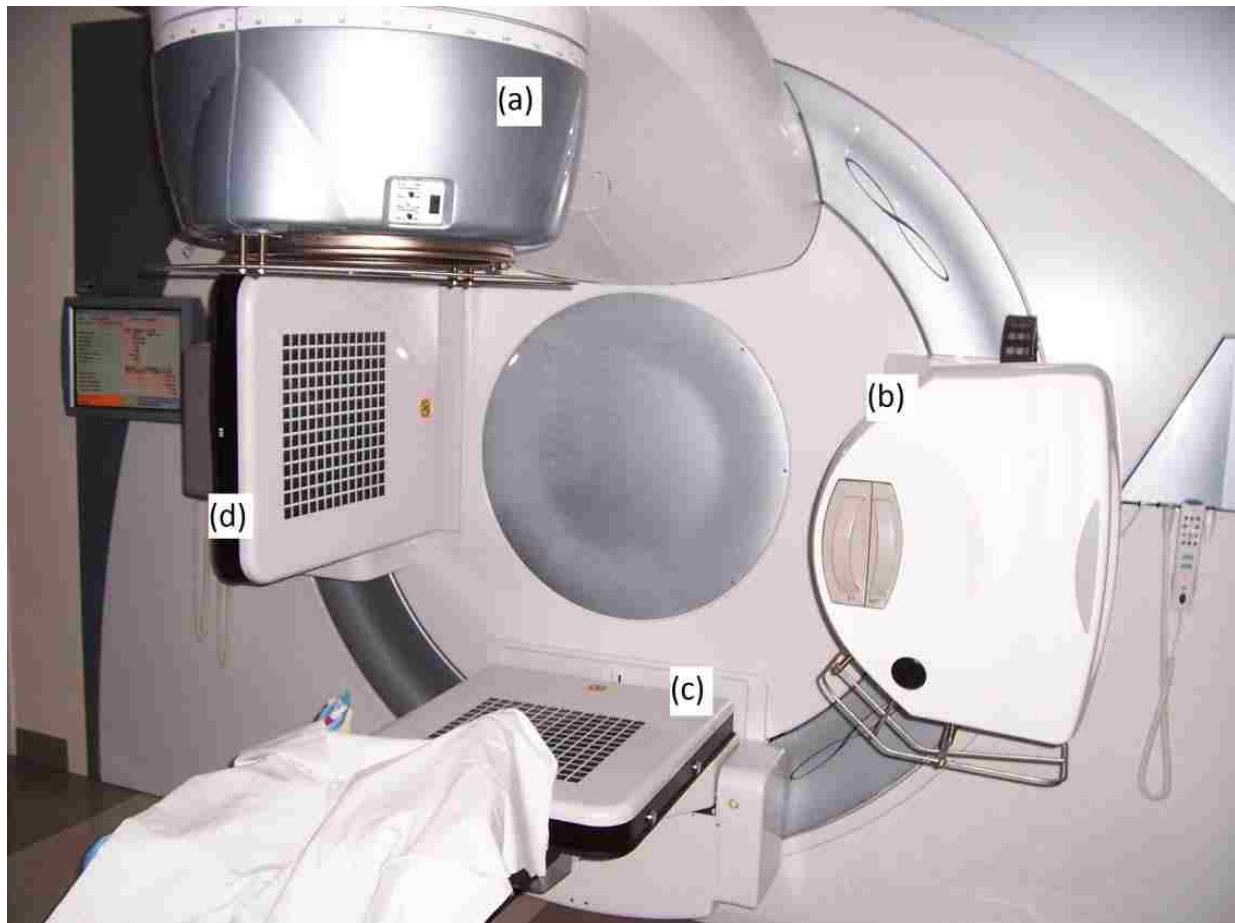
Figure 1.3: Photograph of the Elekta Infinity system with (a) the MV x-ray beam source (linac head), (b) the kV x-ray source, (c) the MV flat panel detector, and (d) the kV flat panel detector.
