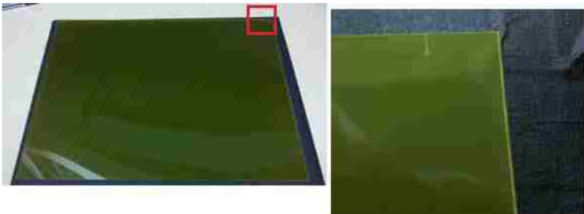
Figure 2.9: (Left) Gafchromic EBT 2 film shown in the landscape orientation. (Right) Enlarged view of upper right corner (red box) showing the slit which distinguishes which side of the film to use.
