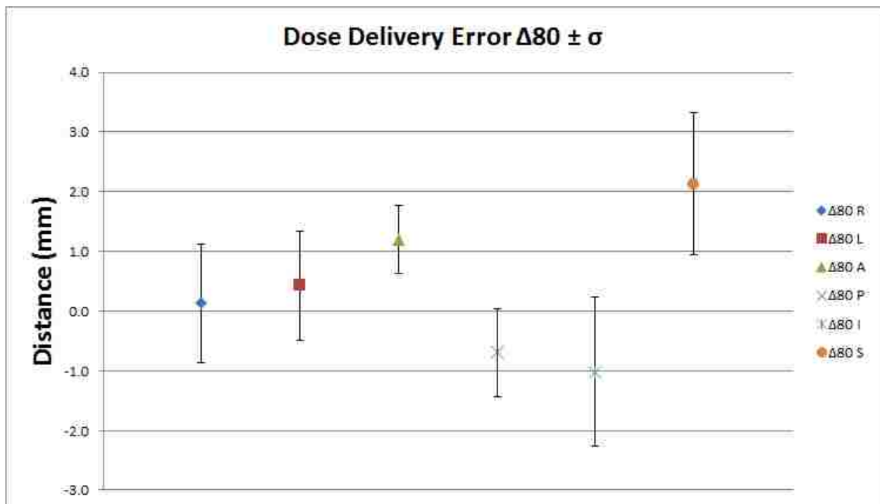
Figure 3.5: Plot of the \Delta 80 results using kVCBCT image guidance. The data points are the mean values, and the error bars represent \pm 1 standard deviation.
