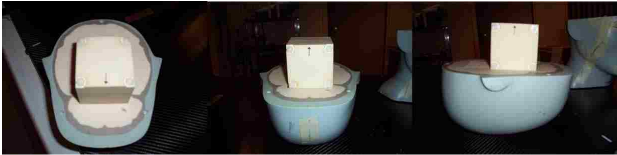
Figure 2.14: The three film cube orientations relative to the phantom anatomy. Shown are the orientations for the transaxial (Left), coronal (Middle), and sagittal (Right) anatomic planes.
