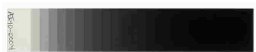
Figure C.2: NIST calibrated TIFFEN Transmission Photographic Step Tablet #2 (The Tiffen Company, Rochester, NY).
