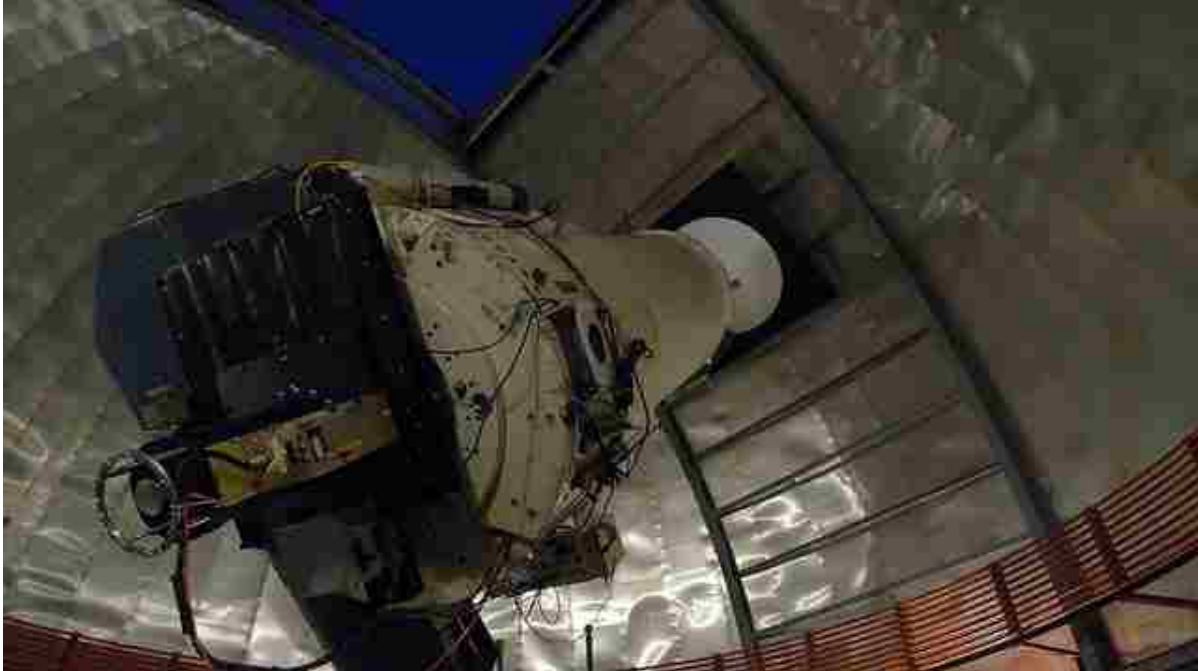
Figure A.3 Flat Screen for Dome Flats. This image shows the 1.0m SMARTS/YALO Telescope at CTIO pointed at the flat screen inside the dome. Note that this picture was taken during morning shut-down, not during dome flats, which is why the dome slit is open.
