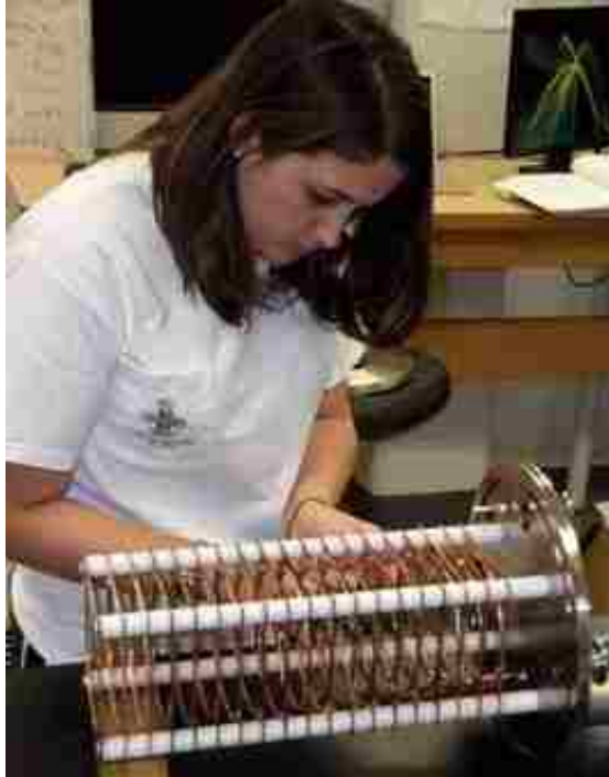
Figure 2-7 A photograph of the grids for the heavy ion recoil chamber being assembled to a NW250 flange.
