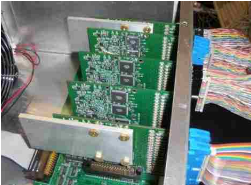
Figure 2-8 Photograph of the ASICs HINP16C system with 5 chip boards installed.
