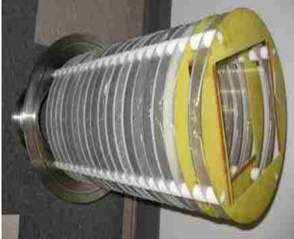
Figure 9-1 A picture of the full heavy ion recoil chamber innards attached to a NW250 flange, complete with two position sensitive circuit boards.
