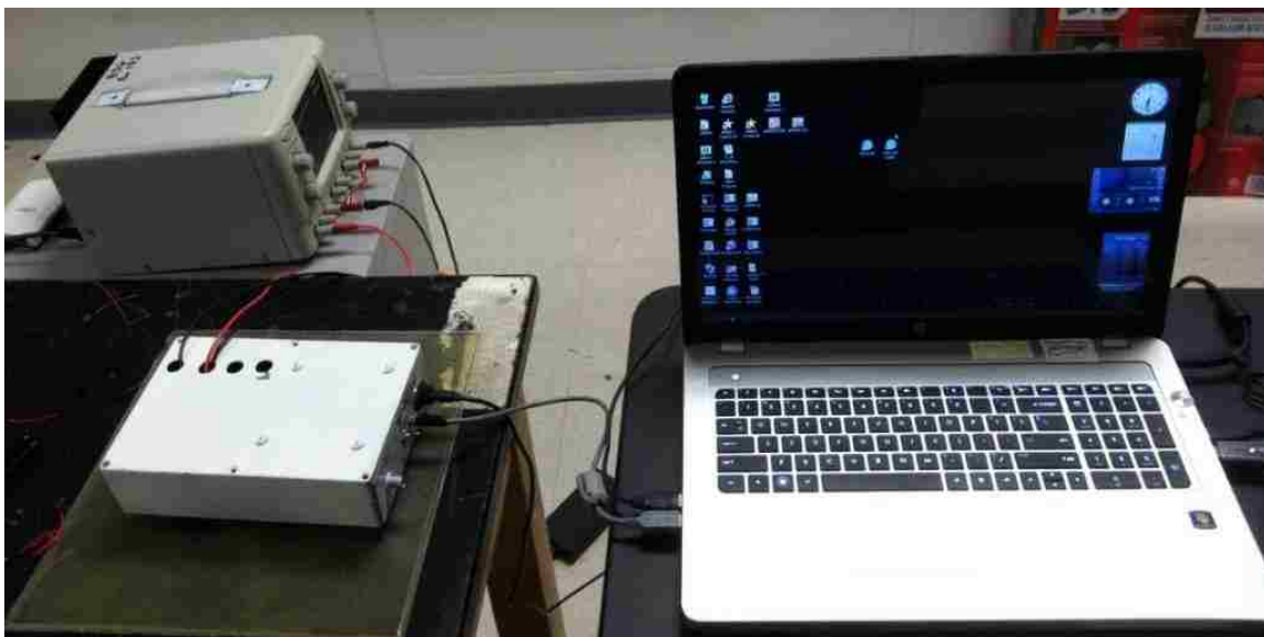
Figure 1.13: Overall layout of qMIDN experimental setup: DC power supply, qMIDN device, and laptop with control software.
