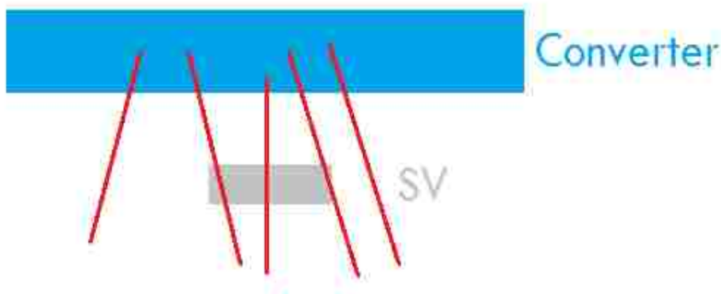
Figure 2.16: Cartoon illustrating MC simulation of the converter layer modeled as a volume source of charged particles.
