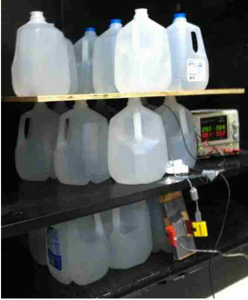
Figure 3.21: Experimental setup for increasing the number of detected events when using the ^{239}\text{PuBe} neutron source. Detector and source are in middle layer surrounded by ring of water jugs.
