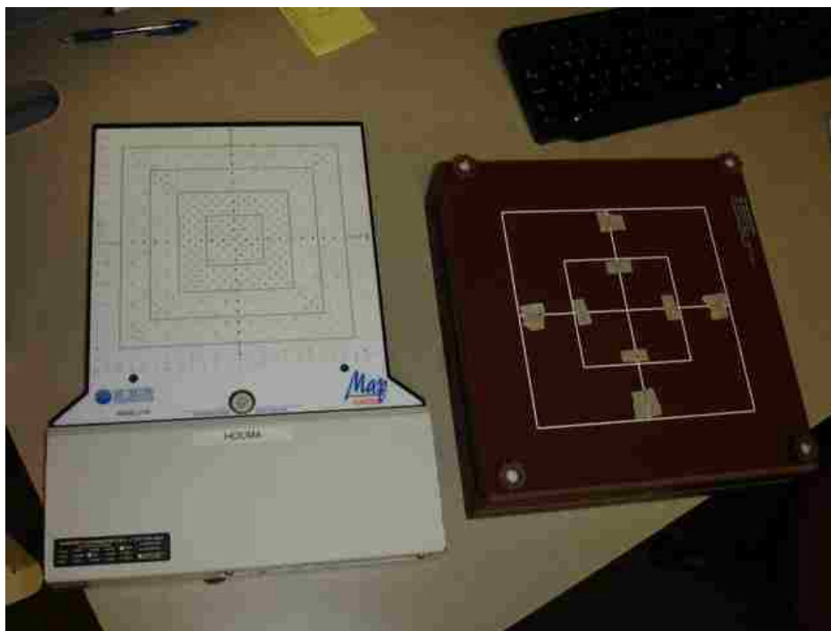
Figure 2.11: MapCHECK device and MapPHAN phantom. The MapCHECK slides into the MapPHAN for rotational delivery measurements.
