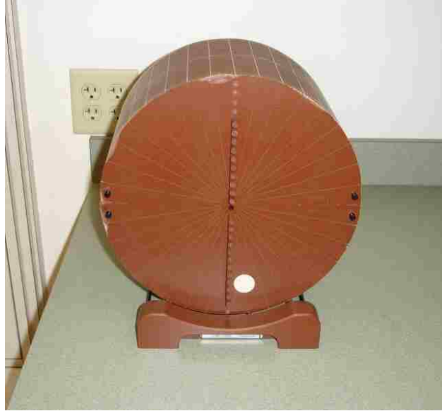
Figure 2.6: Cylindrical “cheese” phantom
