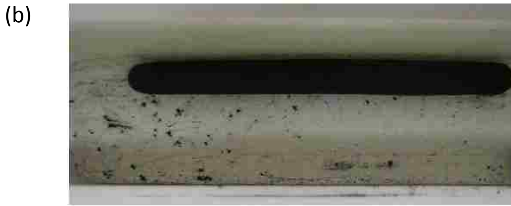
Figure 3.1 (a) Procedure of heating initial powder mixture in tube furnace. (b) Picture of a pressed polycrystalline feed rod with nominal x = 0.1 .
