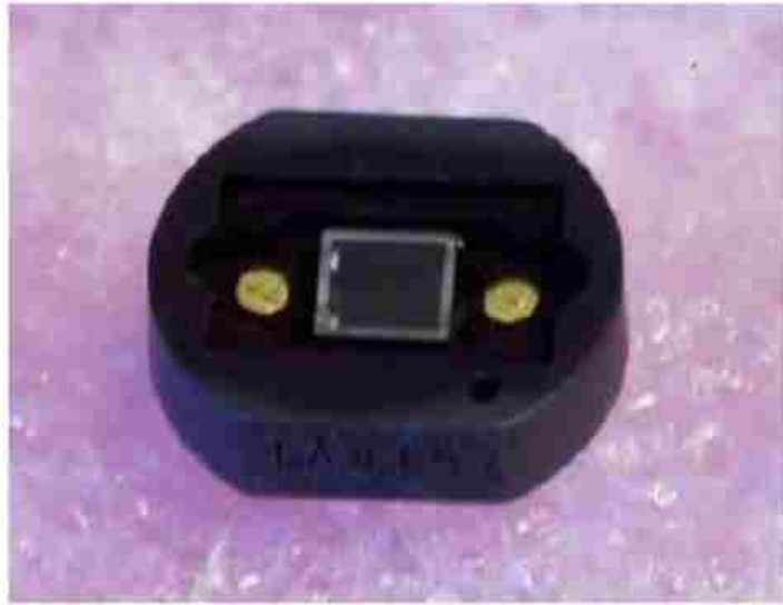
Figure 3.3: The full view of the MPPC is shown in the above photograph.
