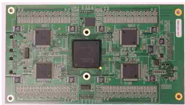
Figure 3.5: The above photo shows a Trip-t Frontend Board used for MPPC signal read out.
