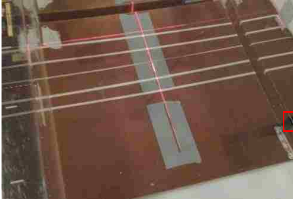
Figure 2-12: Overhead view of the Solidwater®/CT laser alignment. A black, plastic spacer (in red box) was used to immobilize the SolidWater® within the water tank.
