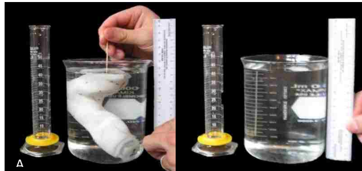
Figure 2-9: Organ surrogate volume measurements via water displacement. (A) Submersion of surrogate rectum structure, water level is recorded from a ruler. (B) Water is added using the graduate cylinder to the same level displaced by the surrogate rectum structure.
