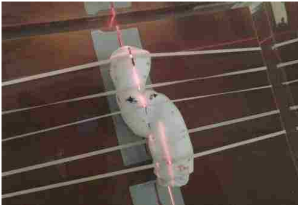
Figure 2-13: Surrogate rectum structure alignment. The structure was attached to the Solidwater® using rubber bands and then aligned laterally with the overhead CT lasers.
