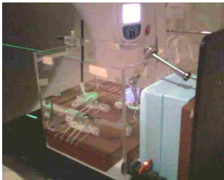
Figure 2-17: Water phantom assembled for scanning on the TomoTherapy Hi-Art II MVCT scanner. This image also shows the bladder attachment arm and the applicator mount.
