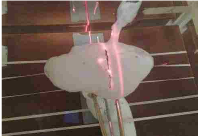
Figure 2-16: Surrogate bladder structure alignment with the overhead CT lasers. Note: a difference in the internal and external overhead CT lasers is seen in this figure. To avoid problems with alignment mismatch between the internal and external CT lasers, all parts of the phantom were aligned to the internal CT lasers.
