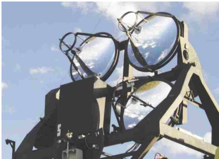
Figure 2.9: The LIDAR system with 3 mirrors that focus back scattered light on the PMTs. The box contains the high frequency laser. Picture taken from [25].
