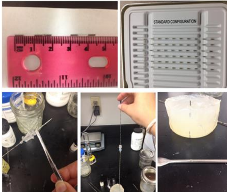
Figure 3.8: Steps for seed implantation. The seed strands before implantation and the needle used for seed implantation.
