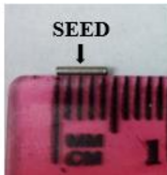
Figure 1.2: Photo of a typical brachytherapy seed (Bard Medical, Inc.) used in permanent prostate brachytherapy. The seed capsule is made of titanium, about 4.5 mm long by 1 mm in diameter as seen on the ruler.
