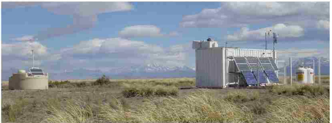
Figure 3.22: The central laser facility, shown with near by surface station “celeste”. The two are connected via optical fibers. From [82].
