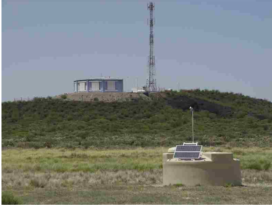
Figure 3.2: A surface detector overlooked by a fluorescence detector at Los Leones, one of the four locations of FD.
