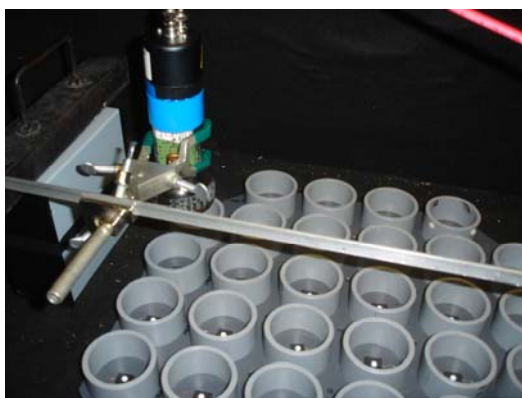
Figure 28. LED setup. The collimated LEDs are being switched on, and light is collected by a PMT.
