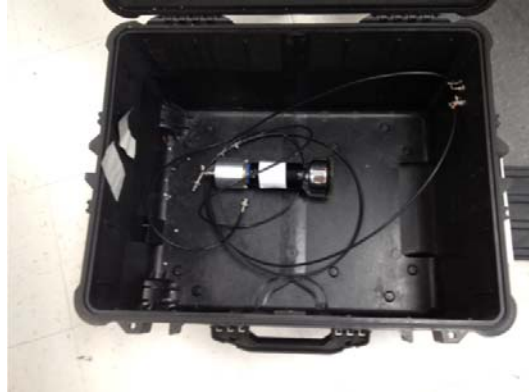
Figure 17. The miniature dark box for testing PMT gains.
