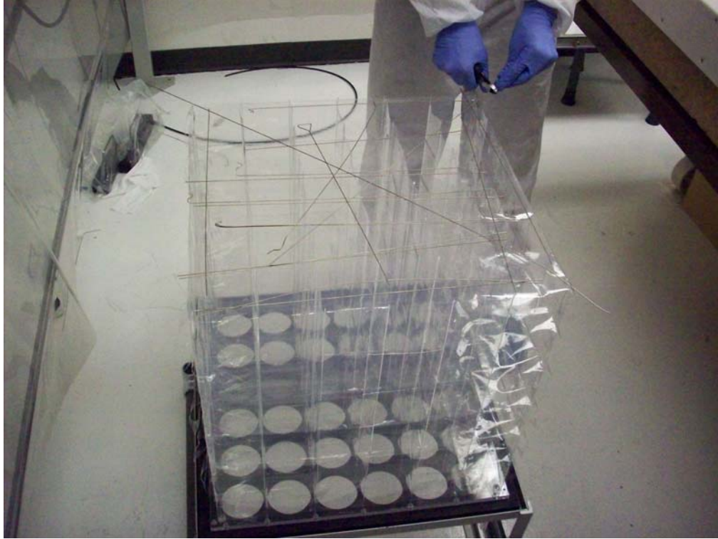
Figure 11. The lattice structure for \mu LENS nearing completion.
