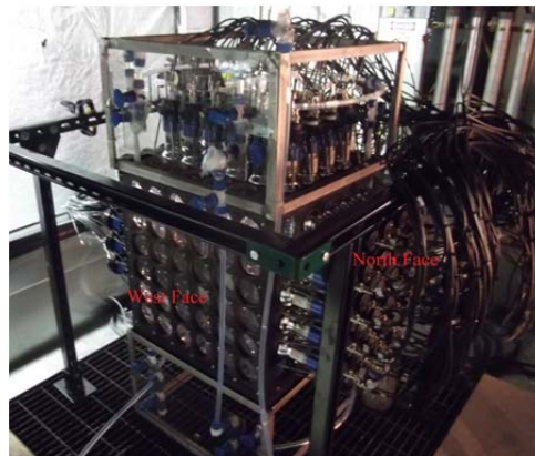
Figure 18. The detector with the PMTs mounted on its surface.
