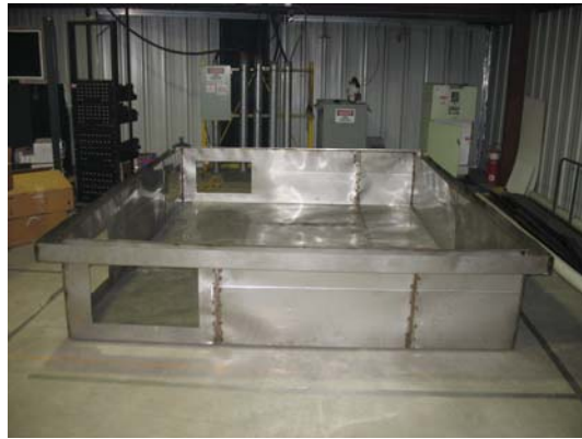
Figure 15. Photograph of the stainless steel base for the Dark Containment.
