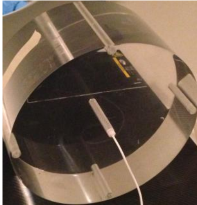
Figure 3: Cylindrical CTDI phantom showing five holes for ion chamber placement
