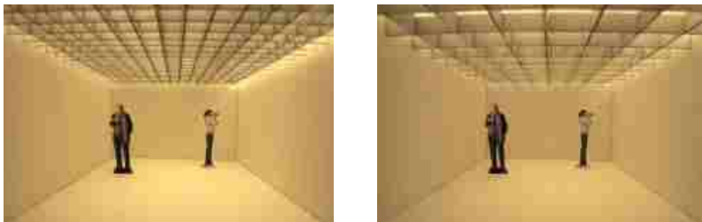
Fig: 7.11 Eggcrate diffuser Study- varying spacing (Images taken in overcast sky box.)
