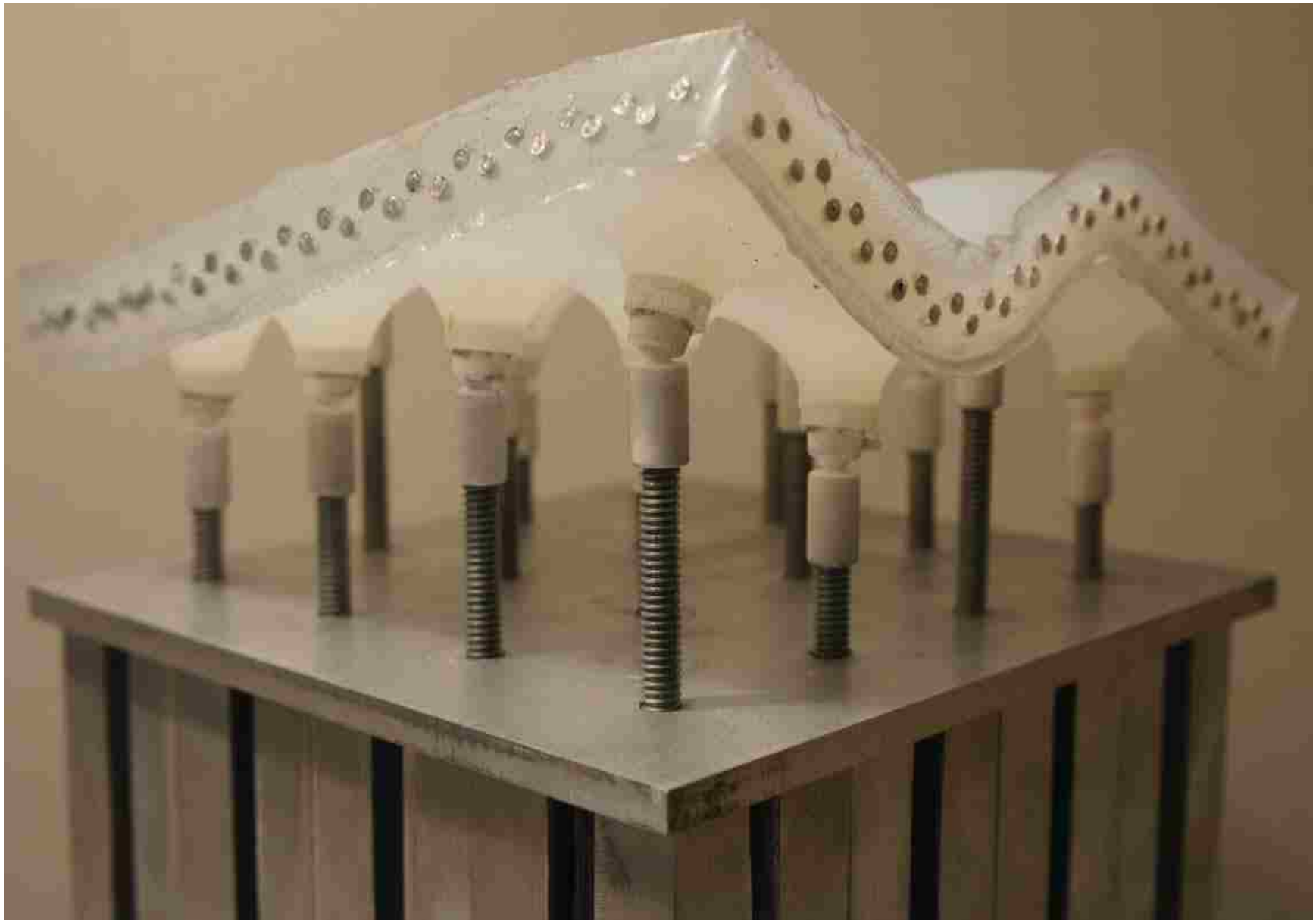
Figure 46: One forming wall from final [m]form prototype
