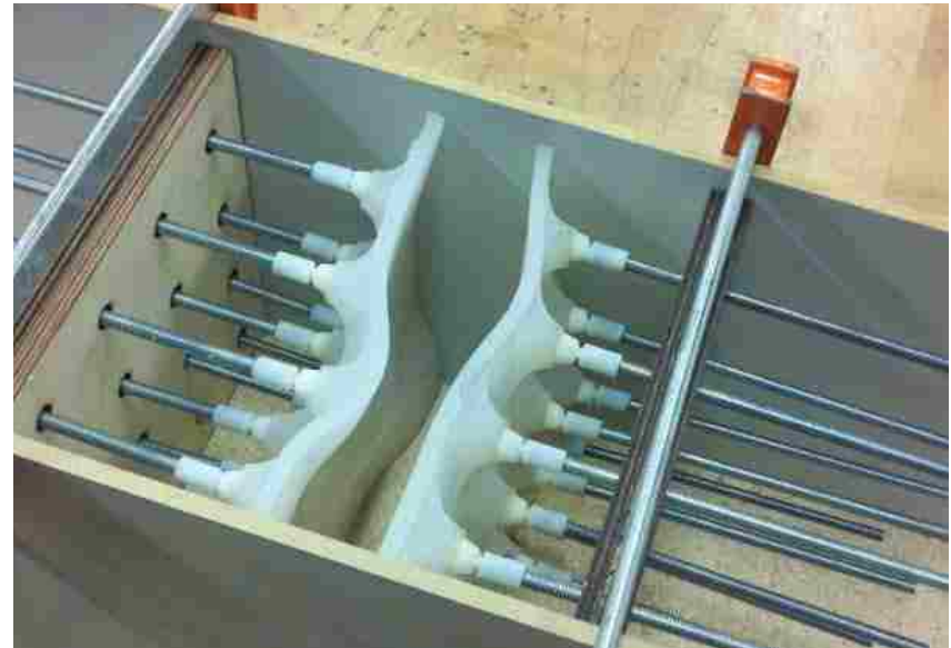
Figure 35: Second full [m]form prototype
