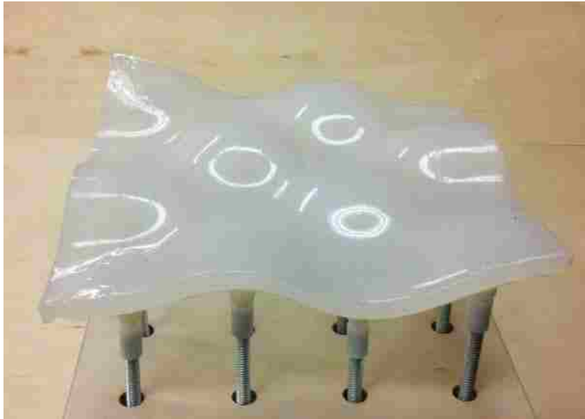
Figure 32: Second [m]form prototype forming membrane and rods
