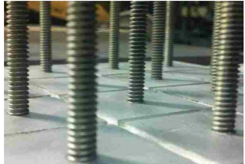
Figure 41: Aluminum wall showing rail guides and 1/4"-20 threaded rods
