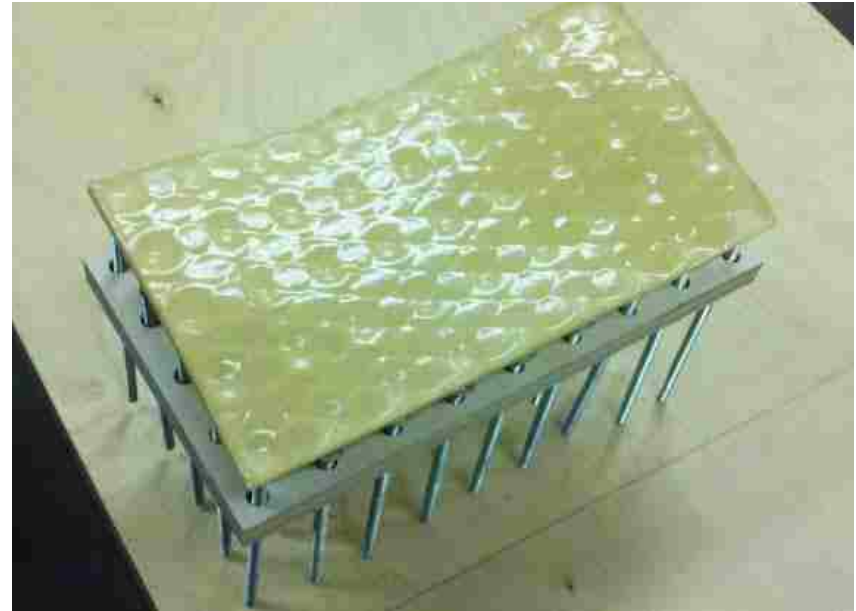
Figure 29: First full [m]form prototype including membrane and forming rods
