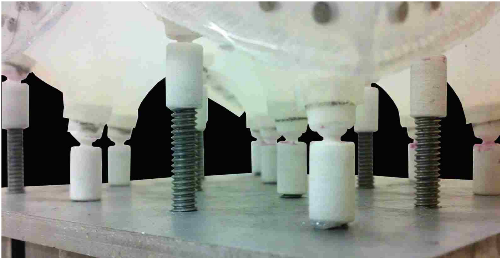
Figure 43: Backside of forming membrane showing 3-D printed nylon ball joints and 1/4"-20 threaded rods extending out of aluminum wall
