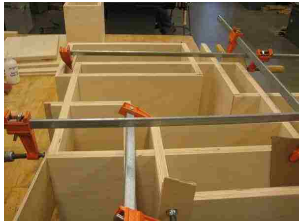
Fig. 9.6 Shelf assembly glue up.
