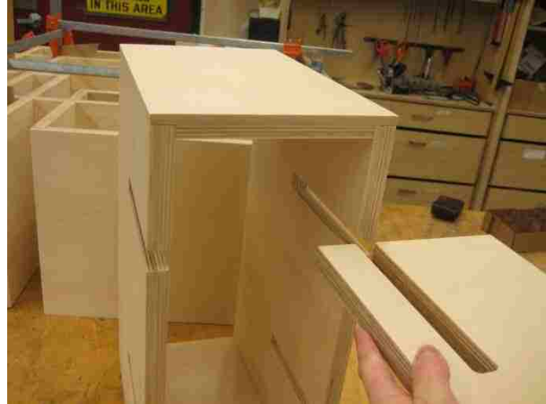
Fig. 9.5 Interlocking slot detail and assembly
