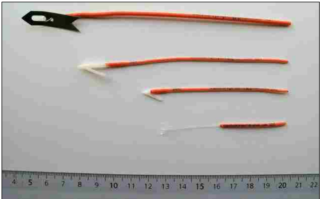
Figure 5.3. From top to bottom, the four tag types used during tagging surveys, stainless steel head dart tag (SSD), plastic tipped dart tags (PDA and PDS), T-Bar anchor tag (TBA).
