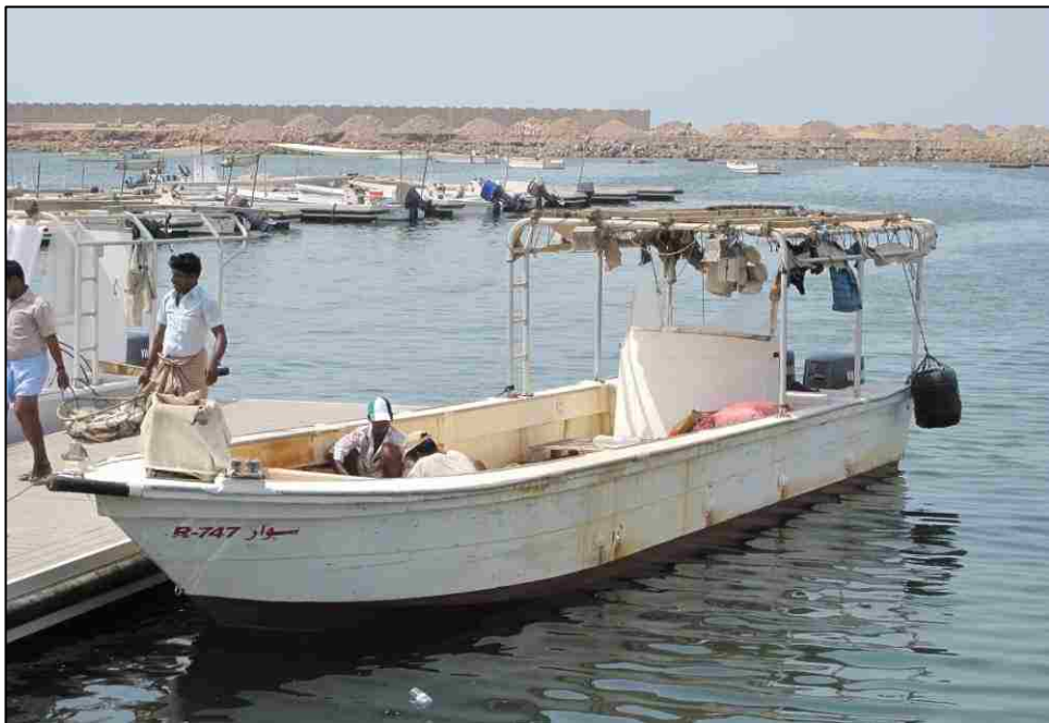
Plate 1.2. The fiberglass vessel, tarad , operating in UAE waters.
