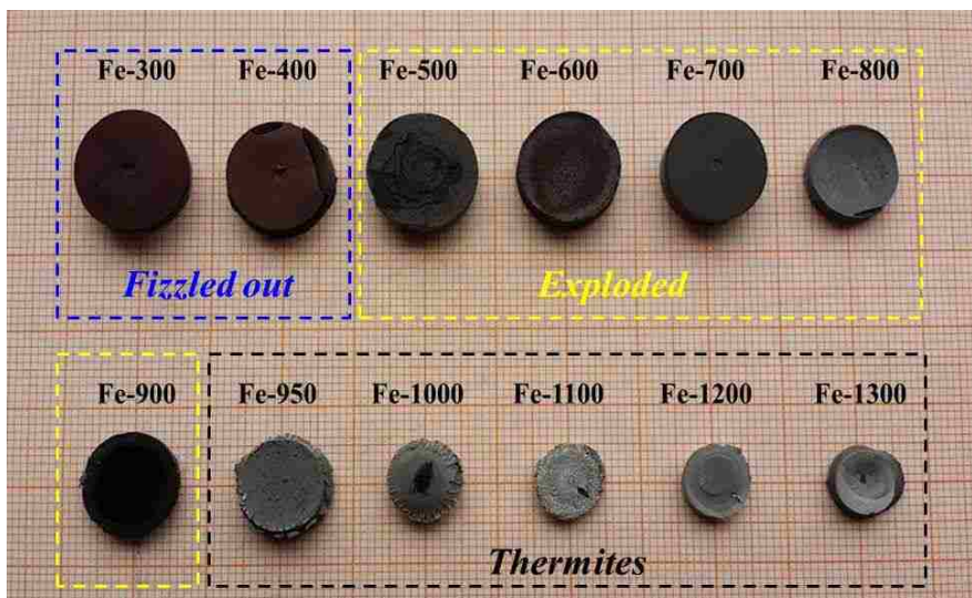
Figure 1. Nanoporous Fe(0) aerogels processed at different final H 2 -reduction temperatures (see Scheme 1). Dashed colored lines group samples that when loaded with LiClO 4 and ignited (Figure 9) fizzled out, exploded or demonstrated thermite behavior. For relative sizes along synthesis, cross-reference with photographs in Scheme 1.
