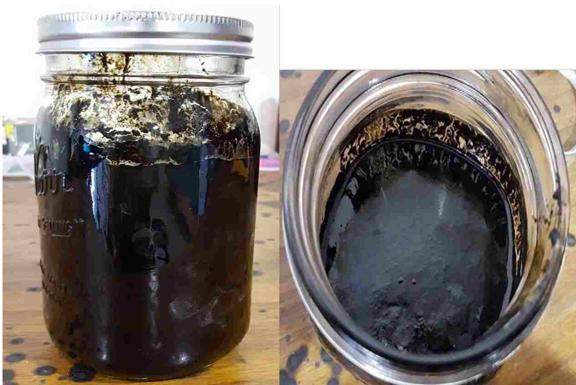
Figure 4.10. Bio-oil collected from the tar collection valve
