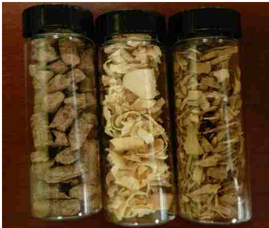
Figure 3.1. Left to right woody feedstocks: pellets, flakes, and chips
