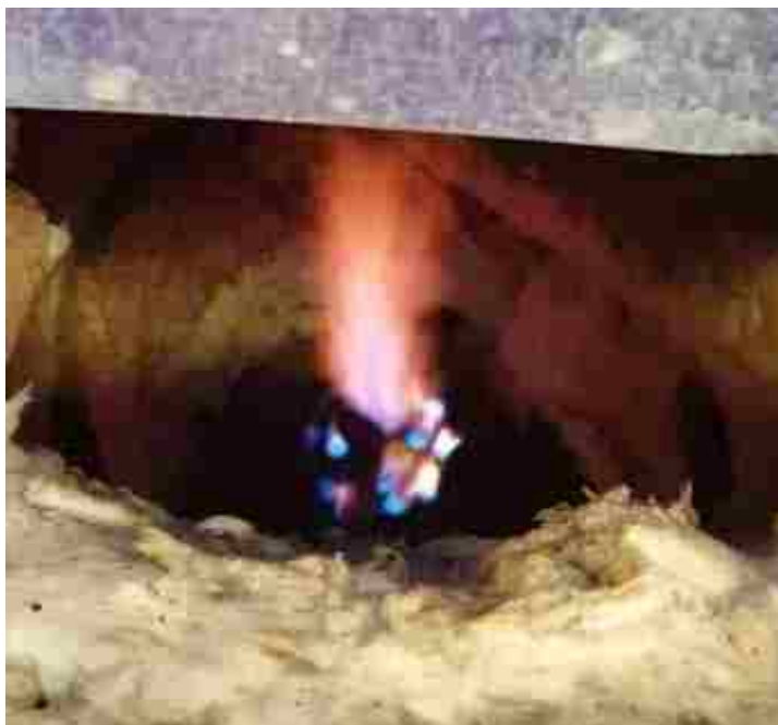
Figure 4.9. Syngas flame inside the combustion flare for 8” reactor
