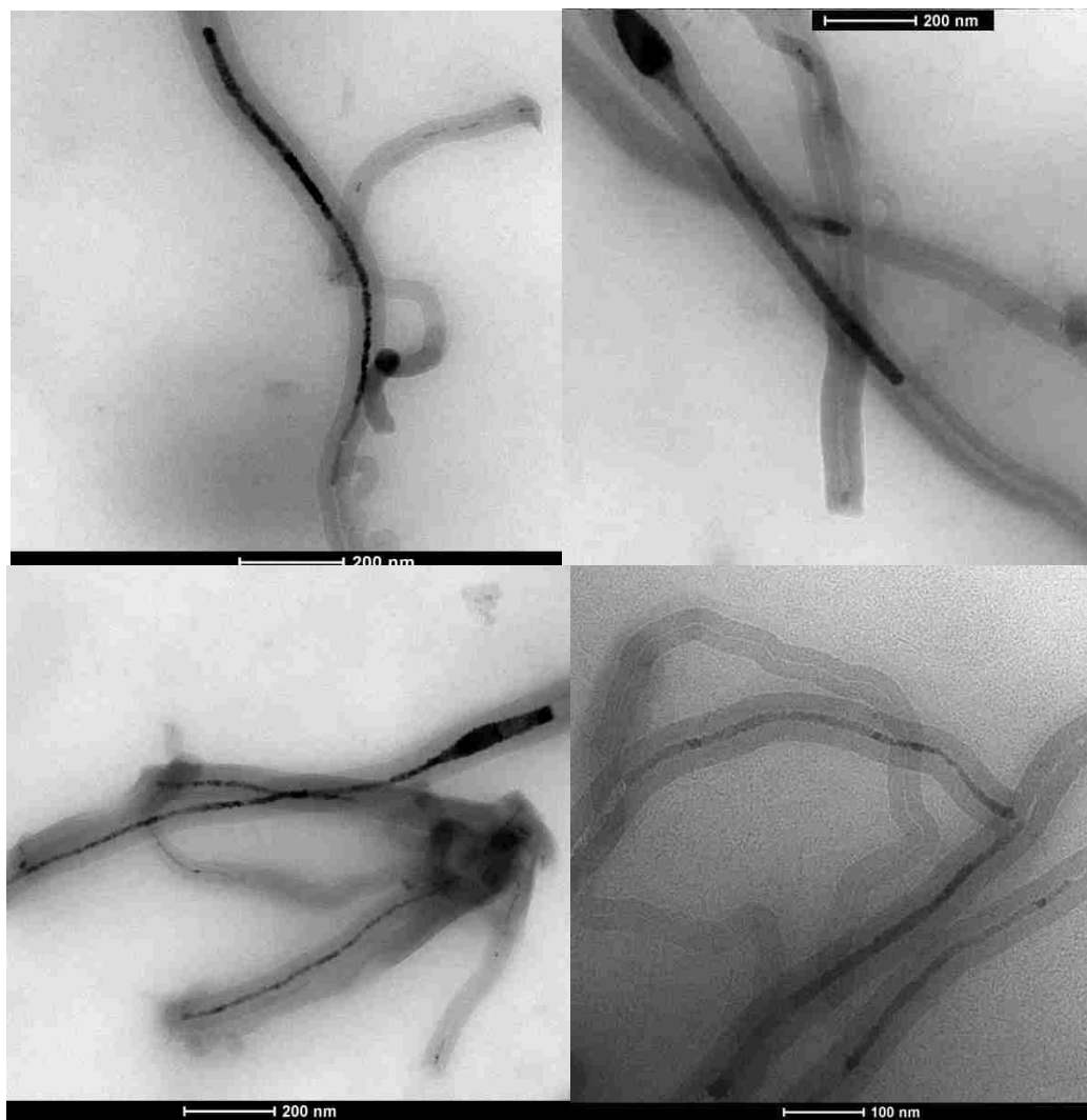
Figure 10.3 STEM images of the nanocables, showing maximum filling of FeSe inside the carbon nanofibers.
