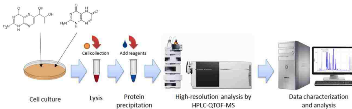
Figure 2. General schematic of the newly developed extraction and quantitative techniques for broad intracellular pteridinic profiling.
