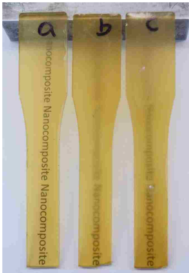
Figure 4. Physical appearance of cured polymers of 2 wt% concentration OMMT as a function of dispersion methodology: (a) sonication in EGS, (b) sonication in MHHPA, and (c) high speed mechanical shear in EGS.
