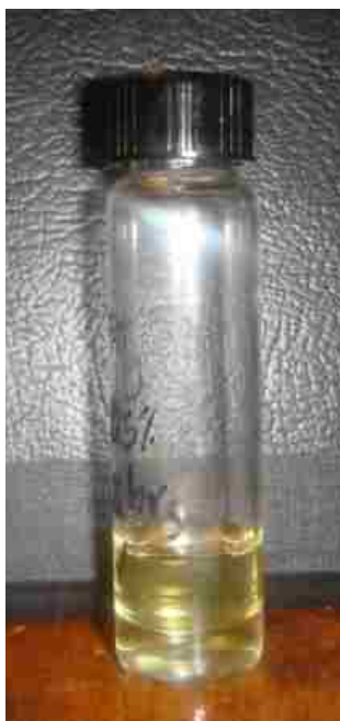
Fig 6: Fatty acid methyl esters (top layer) and glycerol separated into two layers in a vial for the small scale reactor after supercritical transesterification.
