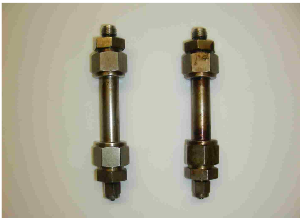
Fig. 1: Mini Reactors used for Supercritical Transesterification Reaction.
