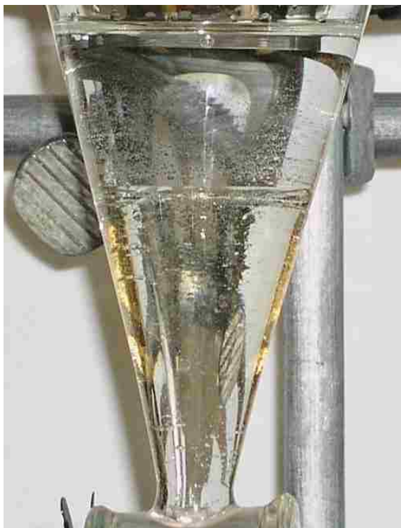
Fig. 3: Soybean oil and methanol (top layer) mixture forming a two-phase system at room temperature before the supercritical transesterification reaction.
