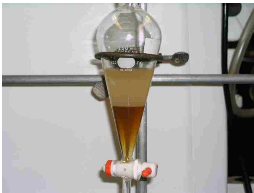
Fig. 4: Fatty acid methyl esters (top layer) and glycerol in methanol immediately after the supercritical transesterification reaction.
