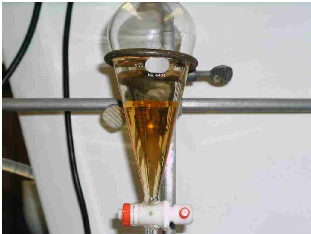
Fig. 5: Non-polar methyl esters (top layer) and polar glycerol separating into two distinct phases, 45 min after the reaction.
