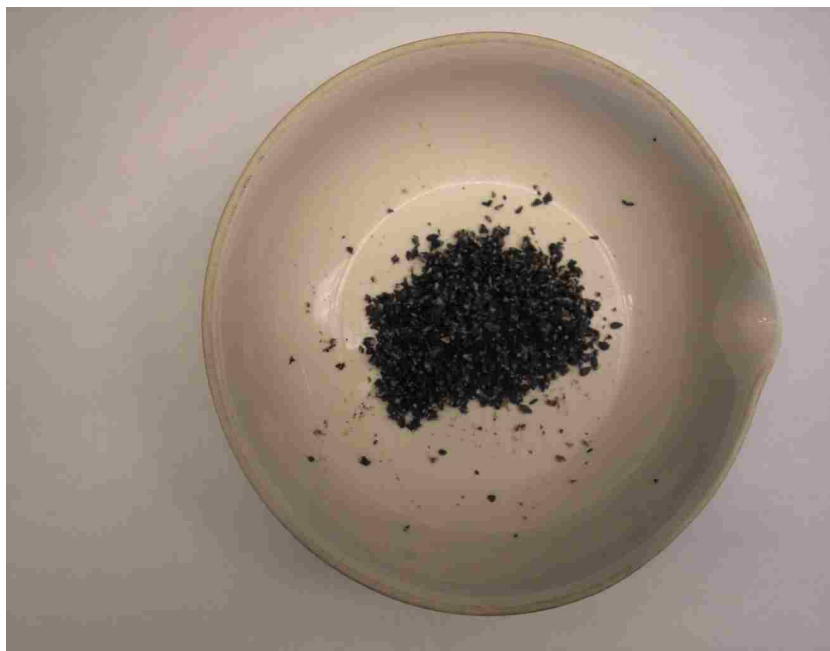
Fig 8: Sesame seeds roughly crushed using mortar and pestle. Crushing the sesame seeds exposes the oil to hexane for easy extraction.
