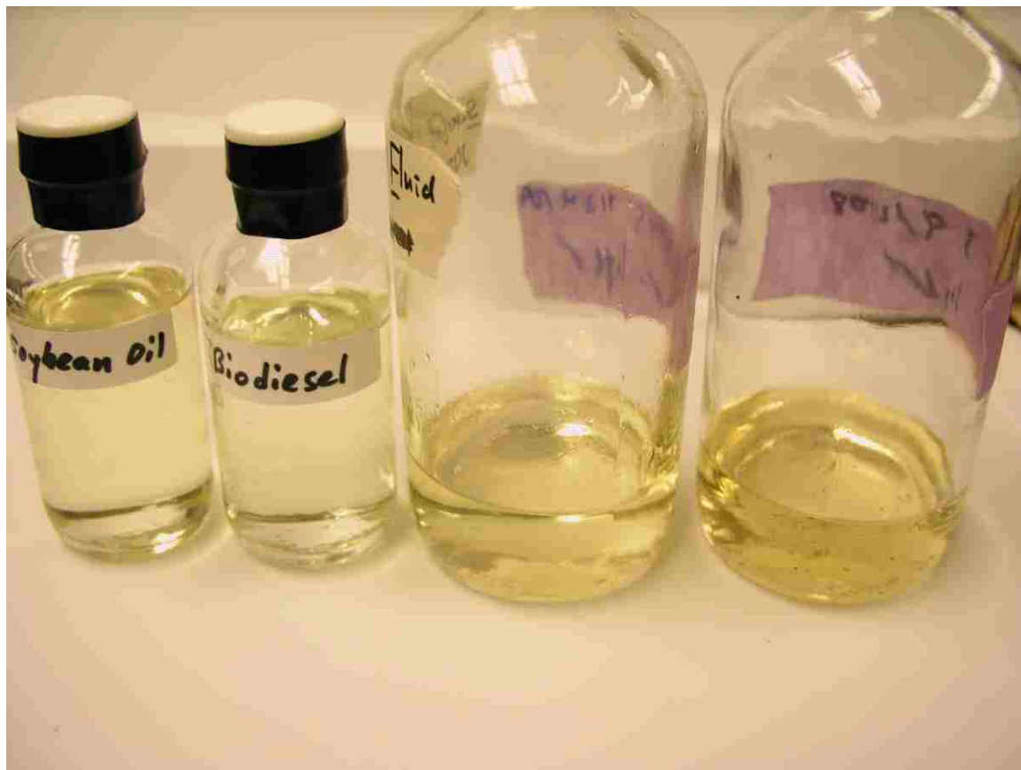
Fig. 1: (L-R) Soybean oil (left), biodiesel from catalyst process, biodiesel (2 nd from right) formed using supercritical methanol, glycerol (right) formed using supercritical methanol
