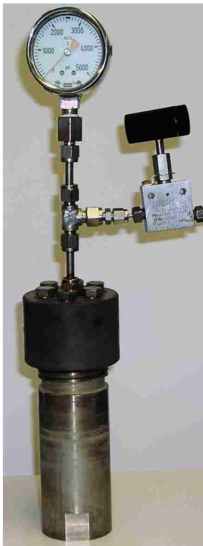
Fig. 2: Supercritical batch reactor is used to produce biodiesel. The pressure gauge and thermocouple are used to determine the reaction conditions. Supercritical methanol and oil are added and heated above 240C and 8.1 MPa using a heating block. The valve is opened to vent the contents if the reaction pressure exceeds 25 MPa
