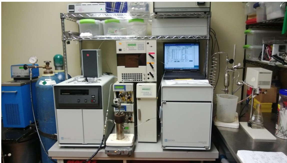
Figure 1. Image of continuous flow reactor use for the carbonic acid hydrolysis of algal biomass
