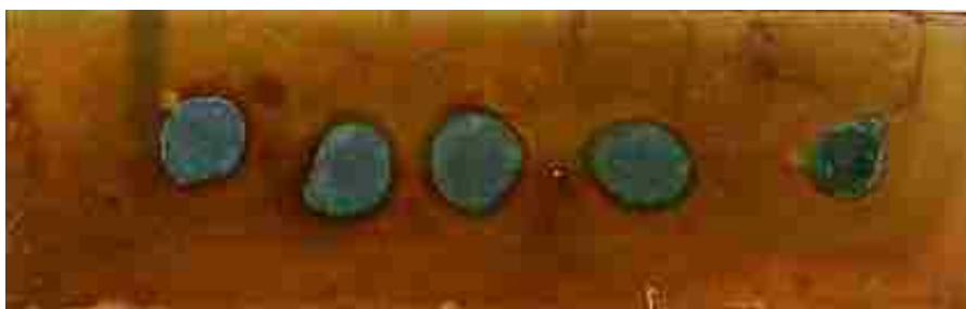
Figure 3.1. Photograph of drop-coated PANI/Au films on Au-coated precleaned glass.
