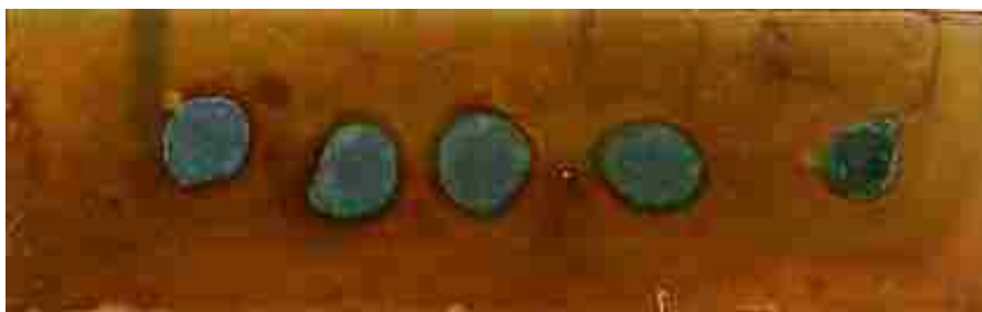
Figure 2.10. Photograph of drop-coated PANI/Au films on Au-coated precleaned glass.
