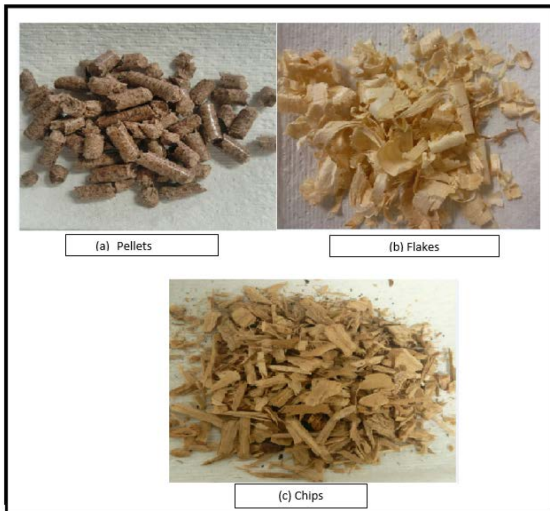
Figure 2-1: Different feed types used in Missouri S&T Energy Center lab.
