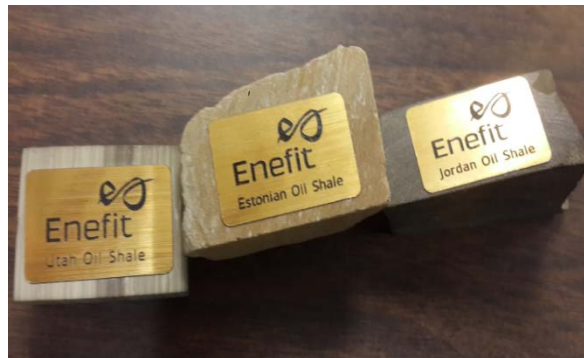
Figure 1-1: Different Samples of Oil Shale at Missouri S&T ERDC Lab. Left to right: Utah oil shale, Estonian oil shale, Jordan oil shale
