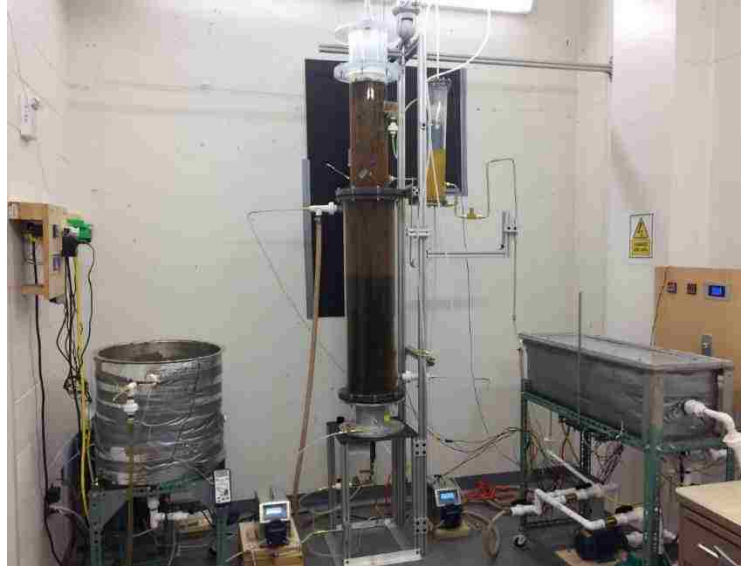
Figure 3. Two-Stages Expanded Granular Sludge Bed Reactor System
