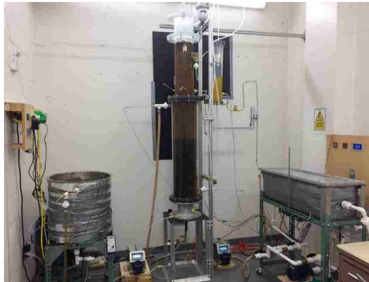
Figure 6. Two-Stage Expanded Granular Sludge Bed Reactor System
