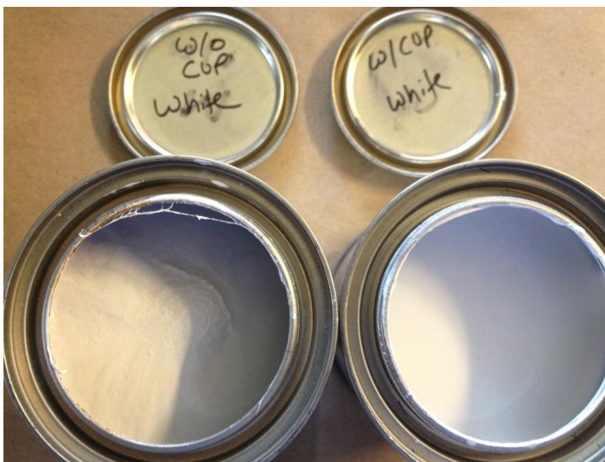
Figure 2. Control and CUP modified paint formulation after 1st freeze thaw cycle
