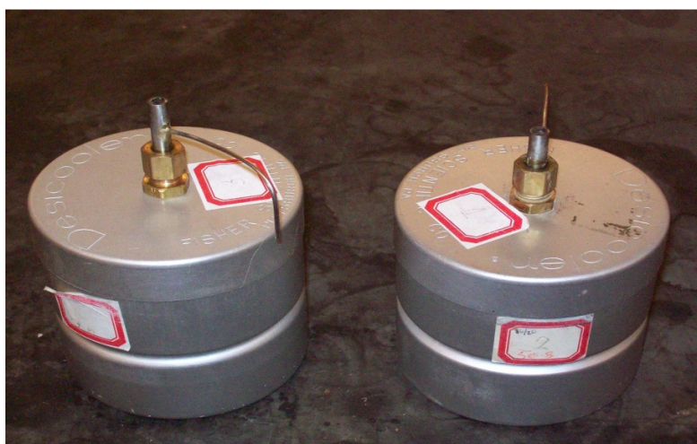
Figure 3.3. Aluminum containers for sonication.
