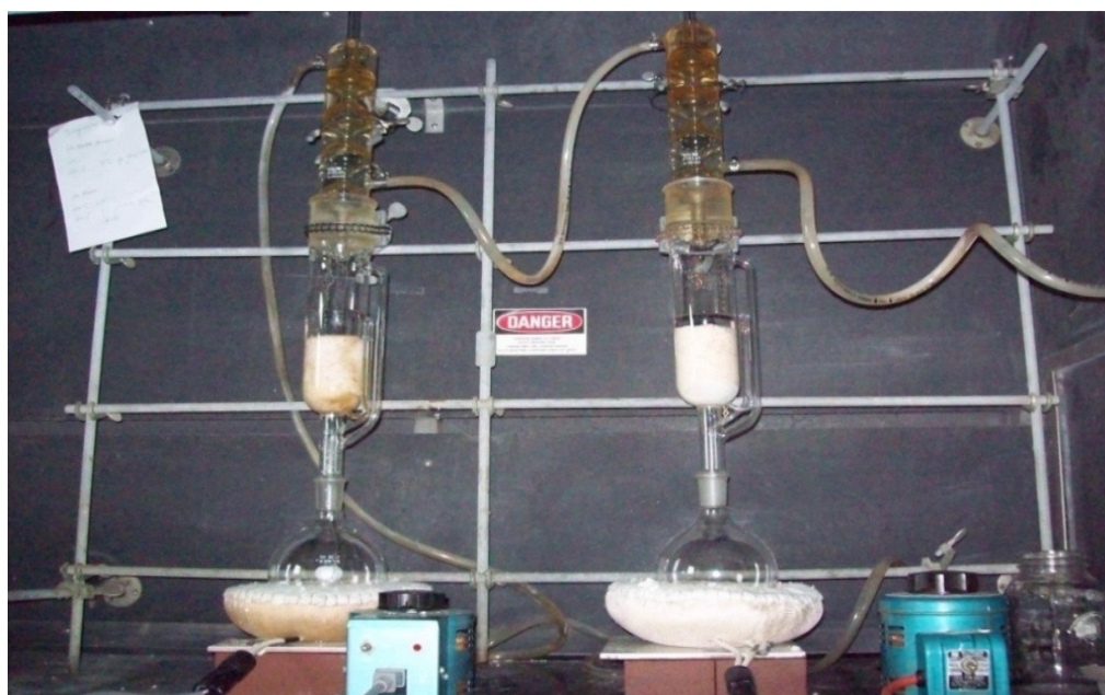
Figure 3.2. A pictorial representation of soxhlet assembly.
