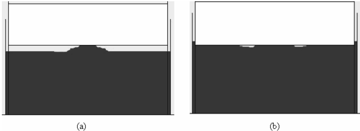
Figure 4.5 Phases - S1818 and Air - Planarization, (a) Before Planarization (0 s), (b) After Planarization ( 1.50 \times 10^{-5} s), (Black – S1818, Gray – Air, and White - Plate)
