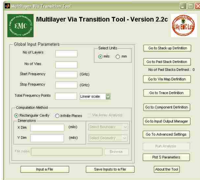
Figure 2.4. Blank 'Main' Window. This window will be used to guide the user through the process of providing all inputs. It is used to access all other windows of the GUI and so is used to control the flow of the GUI.
