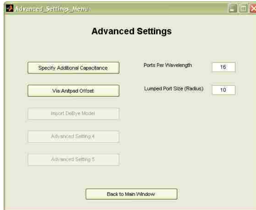
Figure 2.11. Advanced Settings Window. This window provides the user with access to the advanced settings of the tool, like changing capacitance values at an anti-pad, or adding an offset between the via and anti-pad.
