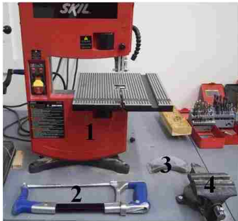
Figure D.2. Setup for cutting sample using band saw. SKIL 9-inch (229 mm) Benchtop 2 Speed Band Saw is indicated as 1. Hand saw is indicated as 2. Safety goggles are indicated as 3. Vice grips are indicated as 4
