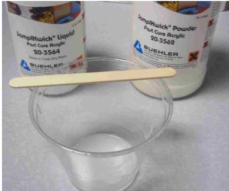
Figure D.8 Mixing powder and liquid for making an epoxy
