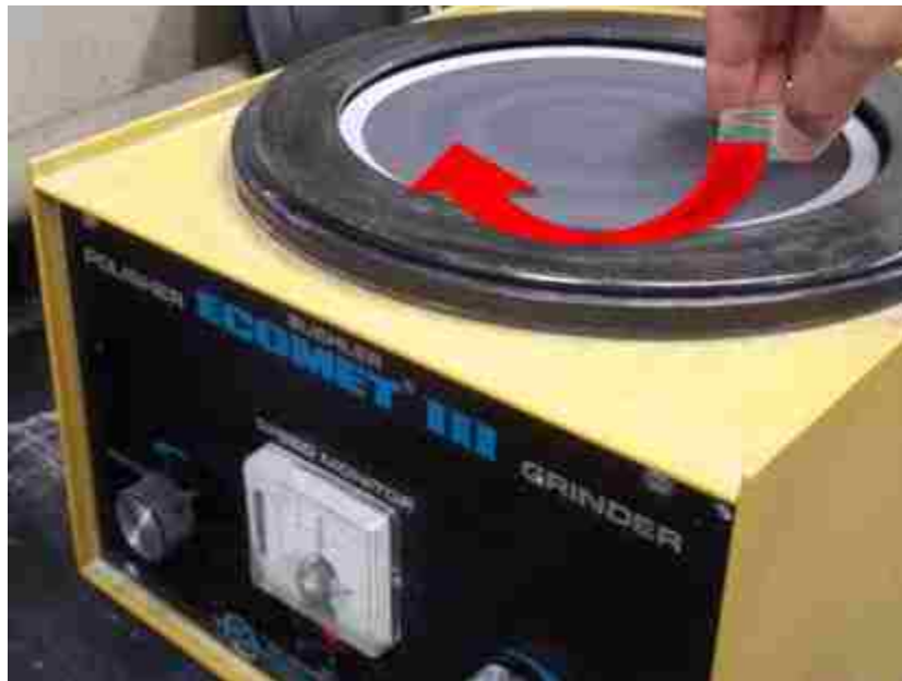
Figure D.16 Example of polishing process. Direction of the sample rotation is indicated with red color.
