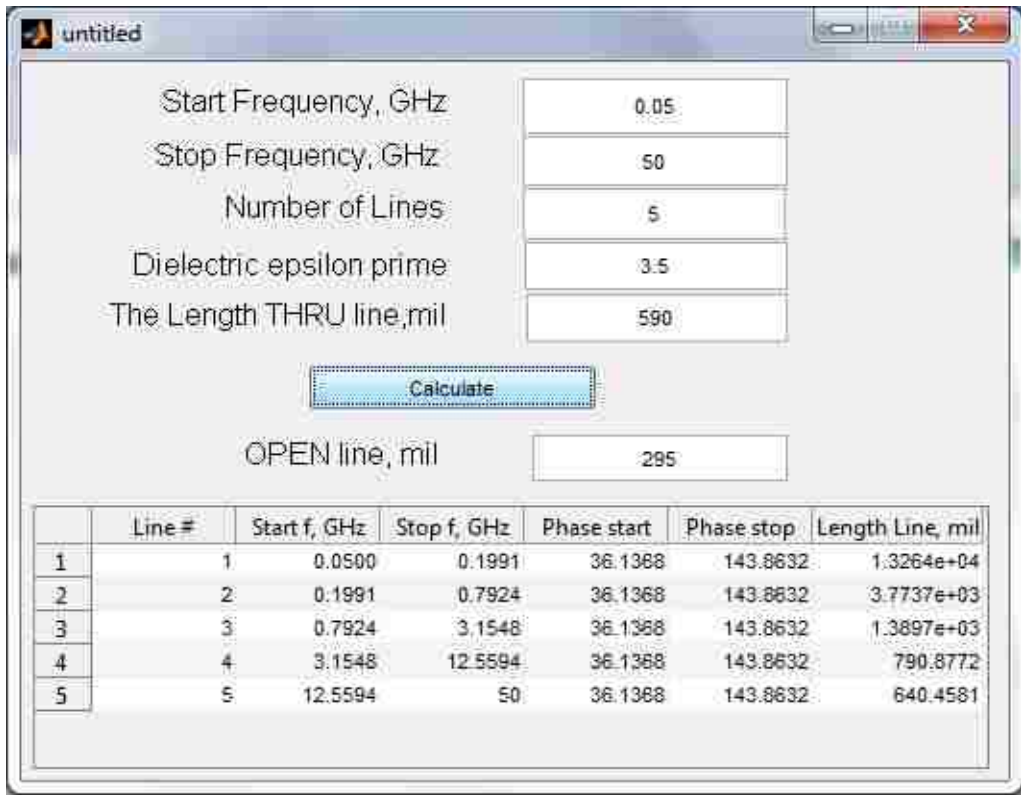
Figure 3.27 Results for calculating TRL calibration patterns for current PCB design using Matlab GUI
