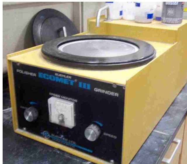
Figure D.13. Buehler Polisher ECOMET III Grinder has been used for polishing
