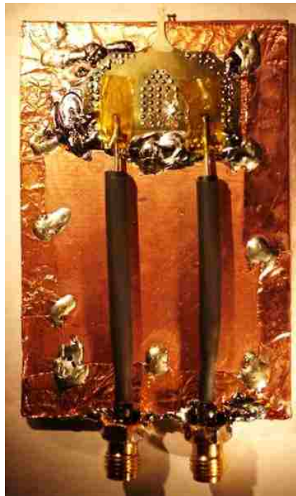
Figure 4.5. The BGA Current Probe Assembly
