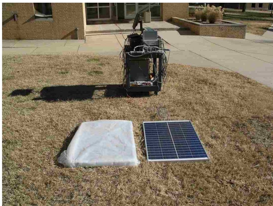
Figure 3.26 Physical shaded solar array with forward converters
