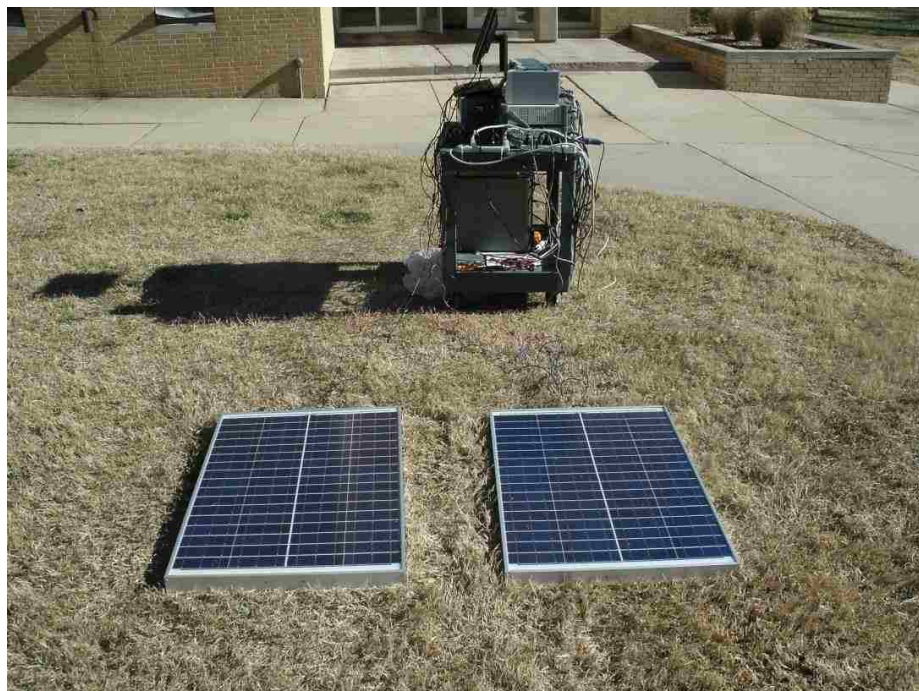
Figure 3.25 Physical non-shaded solar array with forward converters
