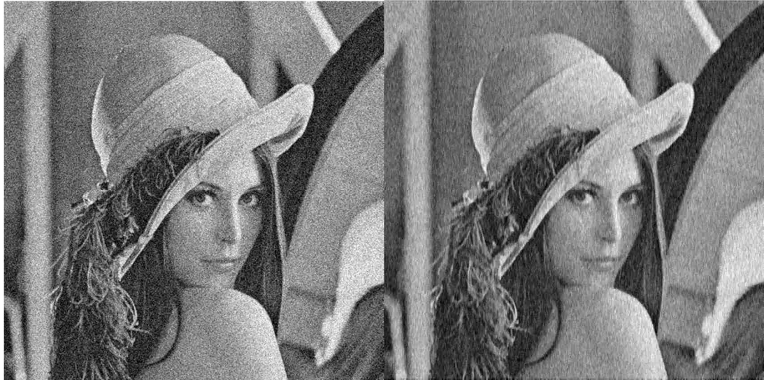
Figure 2.4 Lena image with Gaussian noise (left); median filtered image (right)
