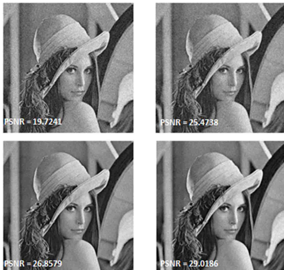
Figure 3.2 Daubechies complex wavelet - Lena image with Gaussian noise (top-left); de-noised version of Lena image with Gaussian noise (top-right); Lena image with Poisson noise (bottom-left); de-noised version of Lena image with Poisson noise (bottom-right)
