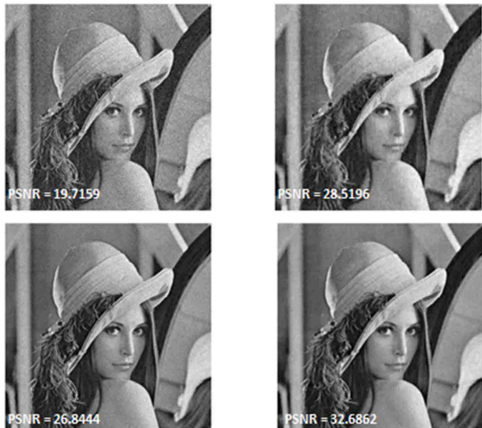
Figure 3.14 IBS and DAMF - Lena image with Gaussian noise (top-left); de-noised version of Lena image with Gaussian noise (top-right); Lena image with Poisson noise (bottom-left); de-noised version of Lena image with Poisson noise (bottom-right)
