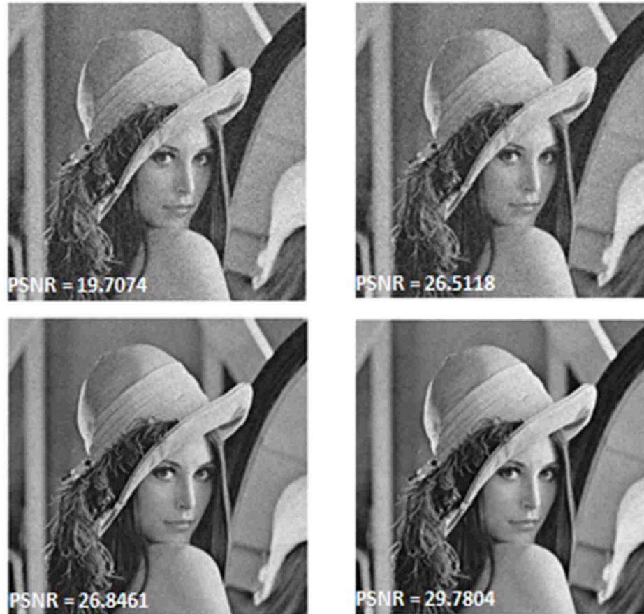
Figure 3.6 Standard deviation estimation - Lena image with Gaussian noise (top-left); de-noised version of Lena image with Gaussian noise (top-right); Lena image with Poisson noise (bottom-left); de-noised version of Lena image with Poisson noise (bottom-right)
