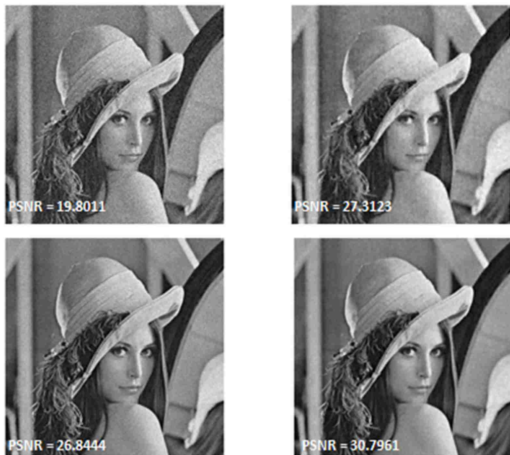
Figure 3.4 Feature-based wavelet - Lena image with Gaussian noise (top-left); de-noised version of Lena image with Gaussian noise (top-right); Lena image with Poisson noise (bottom-left); de-noised version of Lena image with Poisson noise (bottom-right)
