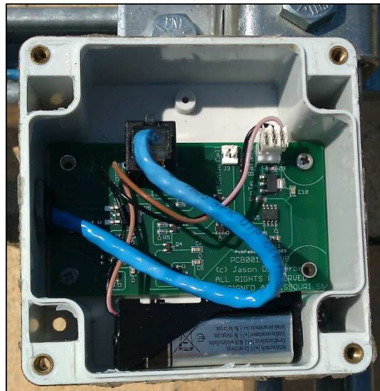
Figure 2.3: Plastic Box to Cover the Sensor and the Solar Cell
