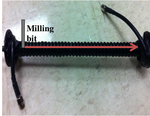
Figure 3.6. Image of a coiled coaxial cable resonator.
