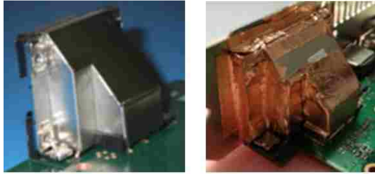
Figure 4.5. Unshielded and shielded DVI connector
