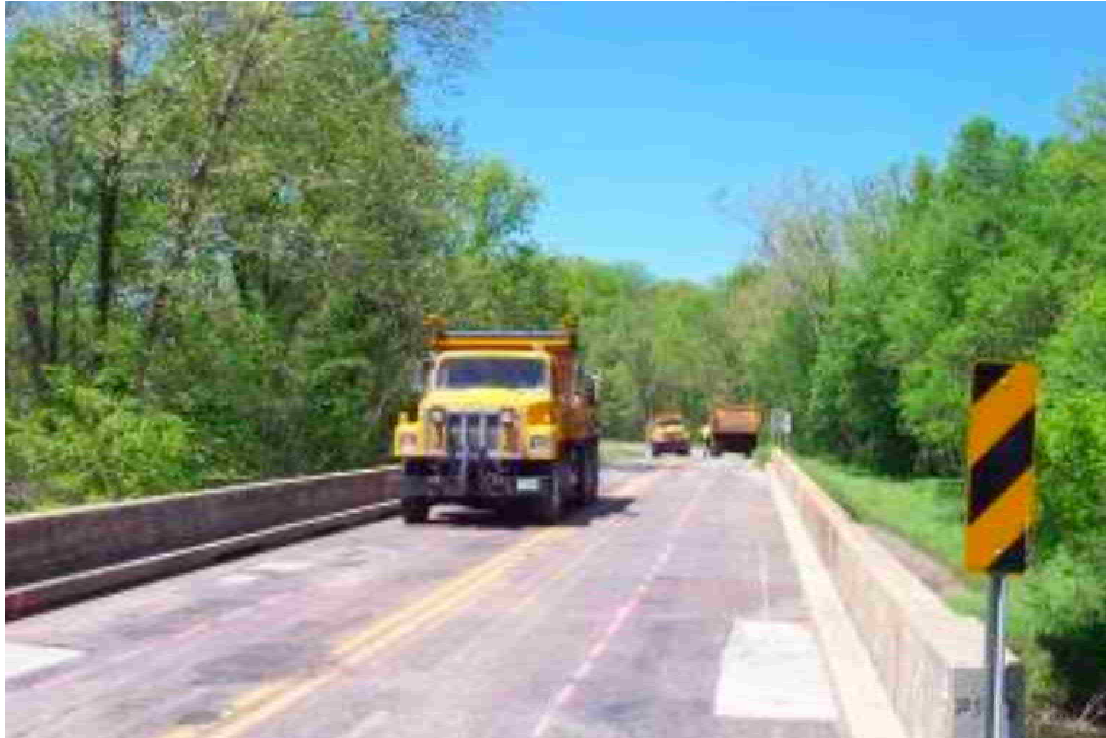
Figure 3.2 - Load test environment with H20 weighted truck.
