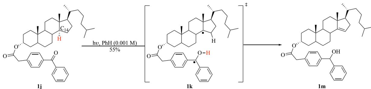
Figure 1.4 Breslow's Photochemical Transfer Hydrogenation
